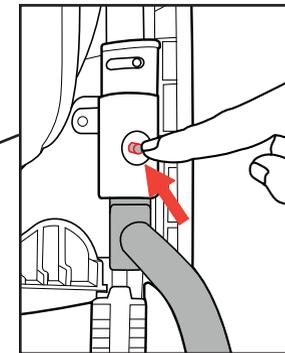
11C. Rotate the Locking Arm down. Repeat for the other side.
