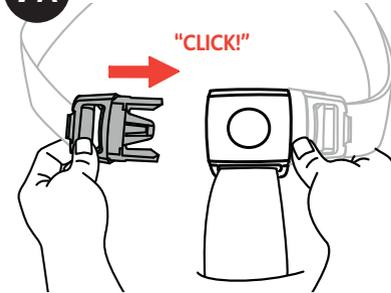
7A. Slide both Waist Clips into the Crotch Strap Buckle as shown. Pull on both sides to make sure the Clips are secured to the Buckle.
