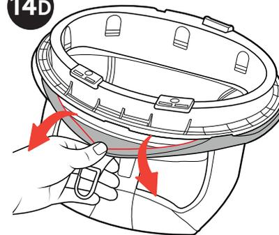
14D. Remove the edge of the Seat Fabric from the Seat Frame.
