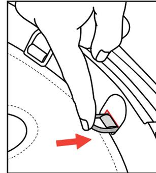
14C. While pushing the ring through the opening on the Seat Frame, at the same time, pull the strap from the opposite side of the opening. Next, remove both rings on either side of the first ring. Alternate removing a ring from each side until you have removed all of the rings.
