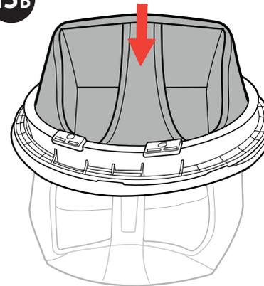
13B. Hold the Child Seat upside down and push the seat fabric down through the Seat Frame. Start with the back edge of the seat, and carefully guide the leg opening wire through the frame. Do not force or bend the leg opening wire while inverting the fabric.
