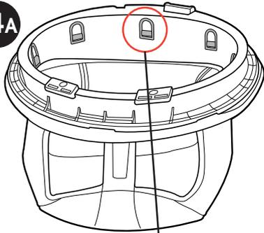
14A. Locate 8 plastic rings on the inside of the Seat Frame.
