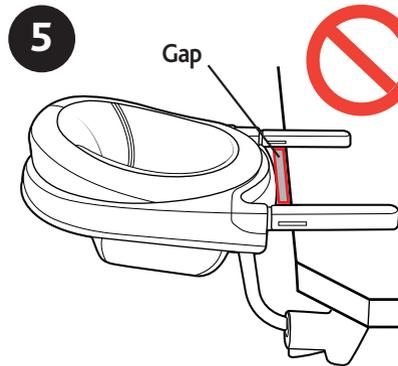
5. Check to make sure there is not a gap between the front of the Hook-On Chair and the edge of the table top.
