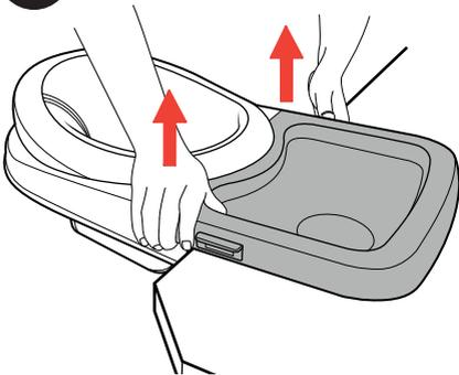
6B. Remove the Tray from the Arms, grasp the Tray on both side tabs and pull up.
