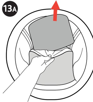
13A. Locate the seat board inside the seat bottom pocket. Lift up on the back edge of the seat fabric and pull out the seat board.
