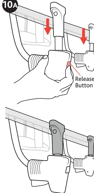
10A. Push in on the release buttons on the front of the Lower Locking Arms to unlock the Clamp Bars, as shown.
