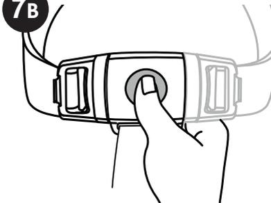
7B. The safety harness can be released by pressing the button on the center of the Crotch Strap Buckle and pulling both Waist Clips out.
