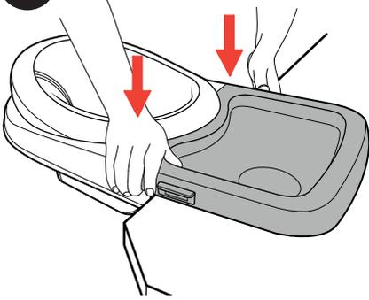
6A. Attach the Tray to the Arms on the Hook-On Chair by lining up the Tray with the Arms on the table. Push down firmly on both side tabs to snap the Tray into place.
