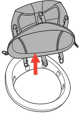
15. Remove the fabric seat covering from the Seat Frame, as shown.
