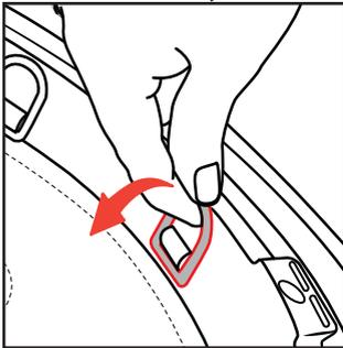
14B. Pull/flip out one of the rings to release the strap.
