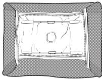
7. Unfold the Bassinet (C) fabric, making sure the metal support rails can open flat. Locate the zipper on the Bassinet fabric and Playard Frame. Attach the zipper sections together starting on one of the long sides, as shown. Make sure the Bassinet fabric is zipped completely around the perimeter of the Playard Frame.
