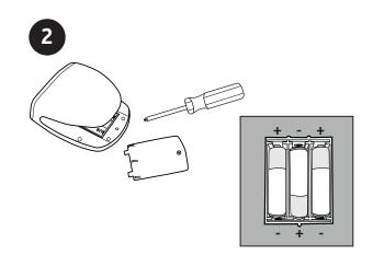
Install 3 "AA" batteries matching the polarity indicated inside battery compartment. Re-attach the battery cover.
