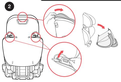
Repeat **Removing Fabric** steps <u>in the reverse order</u>, ensuring that the fabric cover fits onto and around the frame correctly, in particular around the orange belt guides.
