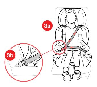
Slide the shoulder belt through the orange Shoulder Belt Guide (A). Make sure belt is below belt guide clip (B).
