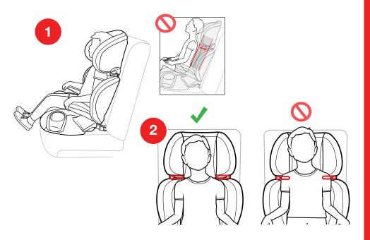
Route the lap belt **UNDER** the 1st Armrest, across the child's thighs, then route the shoulder belt and the lap belt **UNDER** the 2nd Armrest closest to the vehicle buckle as shown. Lap-Shoulder belts MUST be under the **ARMRESTS**, as shown.
