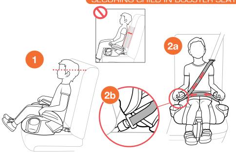
To adjust the Shoulder Positioning Clip, pull the clip up or down to adjust the Shoulder Positioning Clip to be at or slightly above the child's shoulders.
