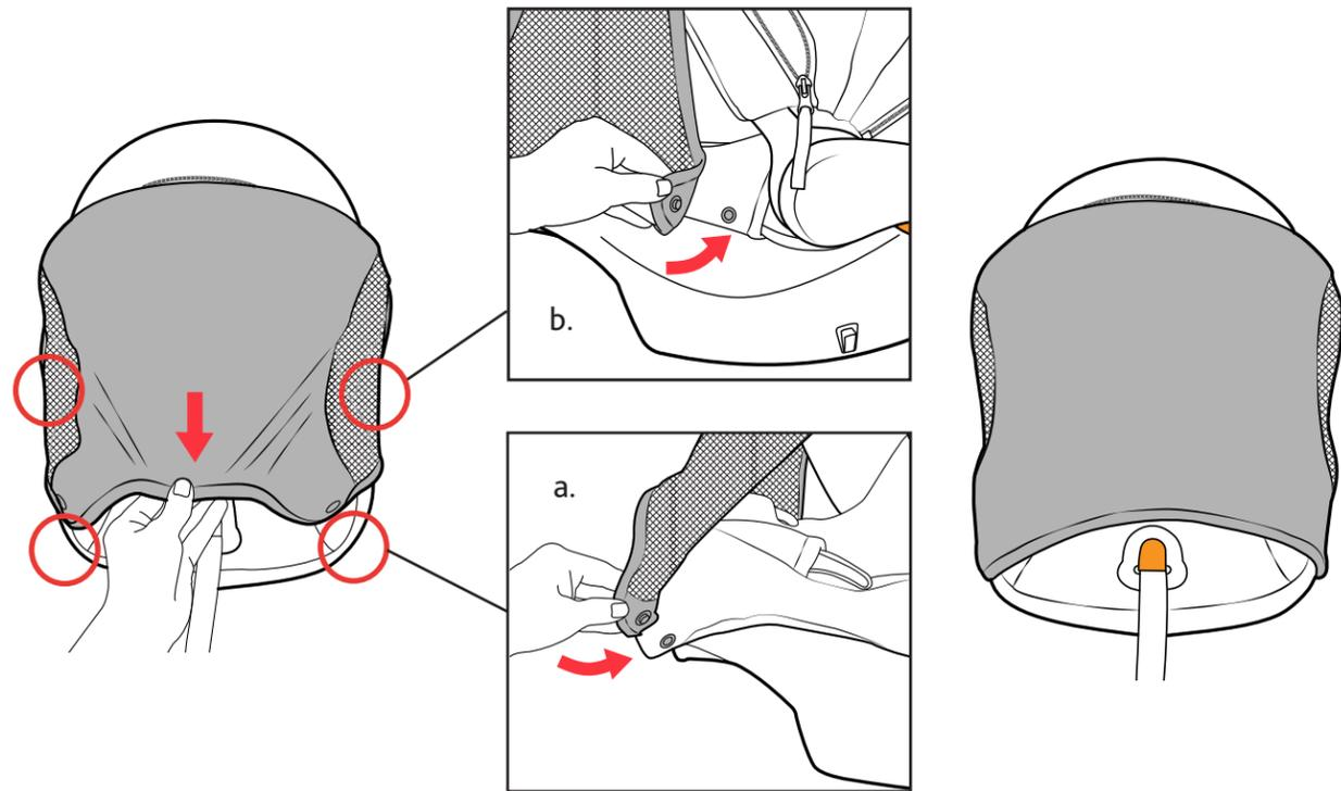
5 Remove the Privacy Shield from the Front Panel section. Pull the Privacy Shield forward, and drape the shield over the car seat. Secure the Privacy Shield using 4 snap buttons. Locate 2 snap buttons (a) on the front corners of the car seat, as shown. Next locate and secure 2 snap buttons (b) below the seat belt guide on each side of the car seat, as shown. Make sure the snaps are always secured. **DO NOT let unsecured privacy shield hang loose.**
