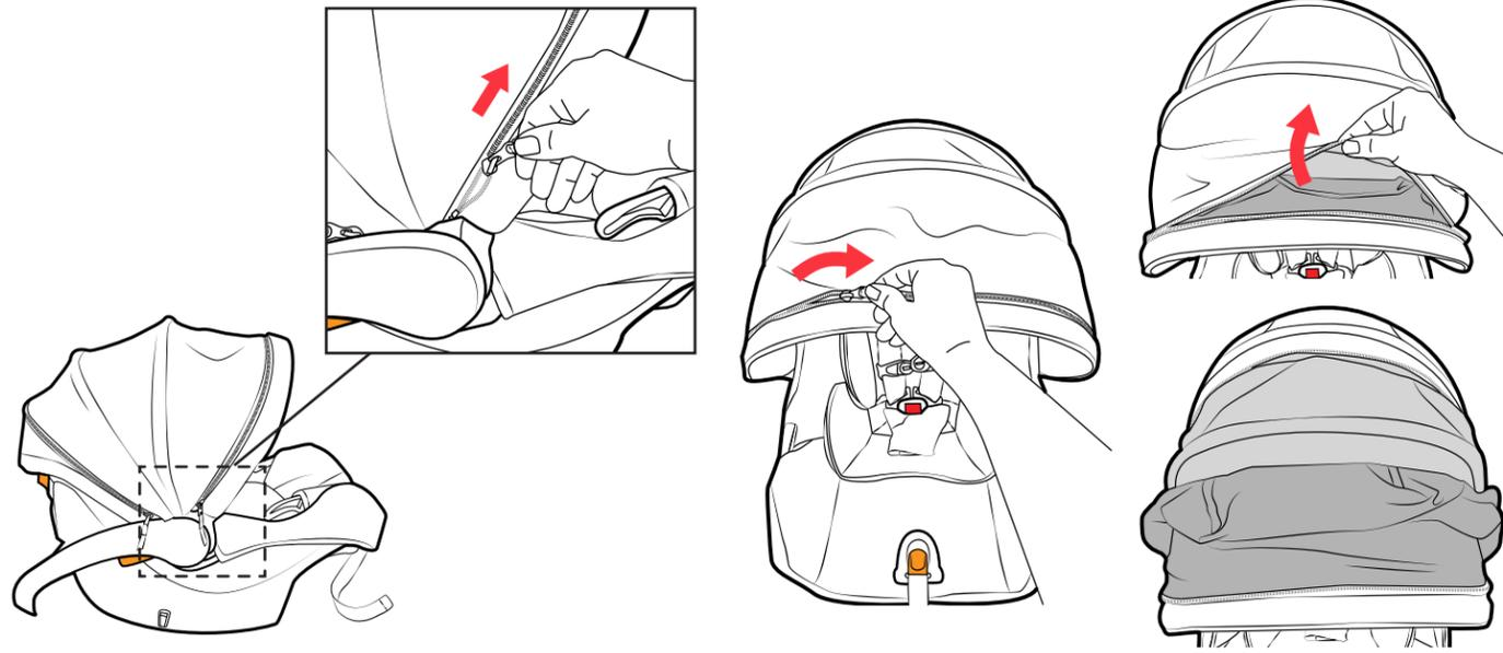
4 With the Canopy fully open, locate the zipper on the Front Panel, as shown. Unzip the zipper and fold back the front panel.
