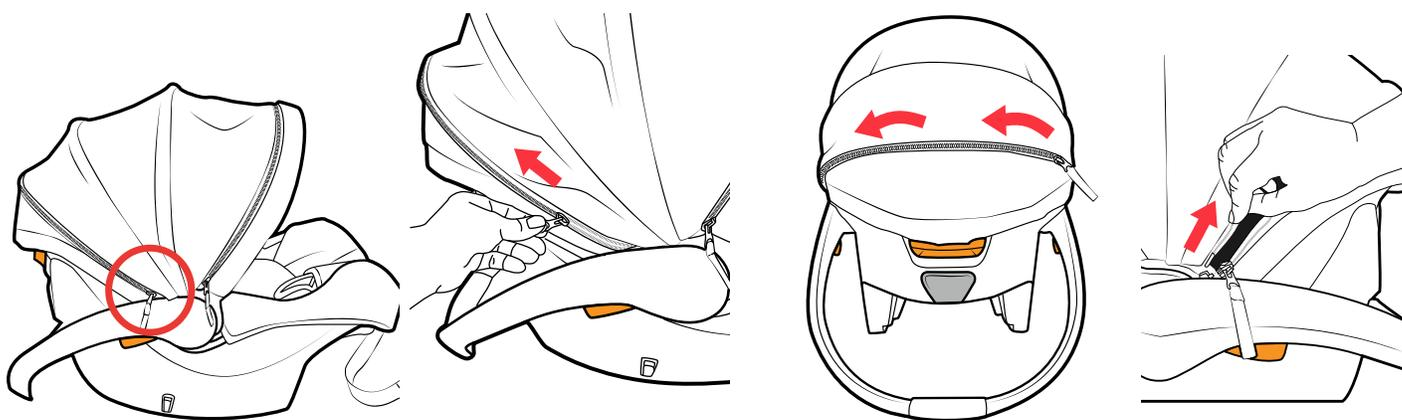
**1** Open Canopy fully and locate the zipper on the Back Panel, as shown. Unzip the zipper slider and remove the zipper pin from the retainer box to separate both sections of the zipper.
