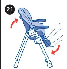
21. Place the backrest in a upright position, and rotate the footrest down.
