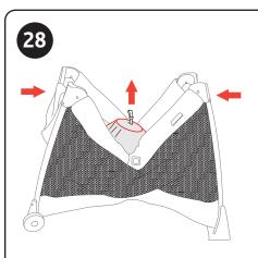
28. Pull up on the center floor hub release strap and pull the playard legs towards the center.
