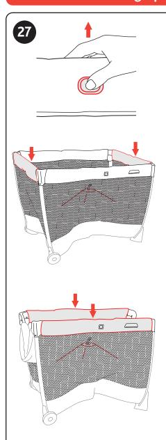
27. Lift and squeeze the Top Rails center release lock, then push down. Release all of the Top Rail locks on all 4 sides. If the Top Rail does not unlock pull up on the center hub to release the floor locks. Center floor hub must be even with top rails.
