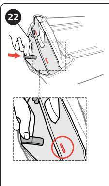
22. Locate the fabric tabs along the outside of the Changing Pad. Thread the fabric tabs through the corresponding openings on the frame and pull the fabric tabs through. Flatten the fabric tabs out to secure them into place. Repeat for both sides.
