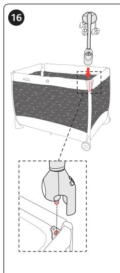
16. Attach the Mobile by sliding the base down over any of the playard corners with the Bassinet attached. Line up the post with corresponding Bassinet corner slot and push down until the Mobile base is completely seated around the corner of playard.
