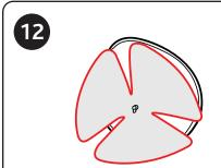
12. Insert the 3 canopy support sections into the fabric sleeve, as shown.
