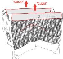
3. The center floor hub must be pulled up to allow the top rails to lock.
