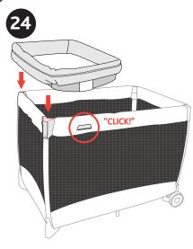
24. IMPORTANT: The Changing Table can only be attached to one end of the playard. Locate the changing table receptacles on the side of the playard. Assemble the Changing Table by lining up the corners of the changing table frame with the corners of the playard. Press down until the changing table latches into the playard receptacles. Pull up on Changing Table to check for attachment. Never use the changer on another surface or playard.
