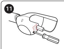
11. Before attempting to operate the Mobile unit, install 3 "AA" batteries. Use a Phillips screwdriver to unfasten battery cover and remove the battery compartment. Insert the batteries and match the polarity indicated inside battery compartment.
