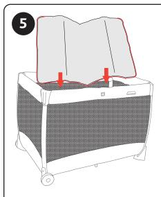
5. Install Mattress Pad, padded side up. Do not use playard without Mattress Pad and make sure to fold hook and loop strap underneath Mattress Pad.
