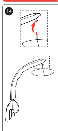
14. Insert the knot at the end of the Toy Mobile canopy string through the opening at the top of the Toy Mobile Arm, as shown. Pull on the fabric to secure the string.
