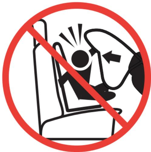
**▲ WARNING! WHEN USING THIS CHILD RESTRAINT, DO NOT PLACE THIS CHILD RESTRAINT IN A VEHICLE SEATING LOCATION WITH A FRONTAL AIR BAG, UNLESS THE AIR BAG CAN BE TURNED OFF.**
