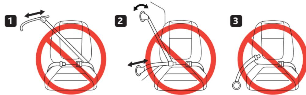
**1. Never use a Lap belt with motorized Shoulder belt.** **3. Never use a Lap-only belt.**
