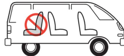
This Booster Seat must be installed in a vehicle seat with a 3-point seat belt (shoulder belt and lap belt). **NEVER** use lap belt only.
