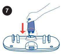
7. Insert the Crotch Bar into the corresponding opening on the tray. Make sure the tether does not hinder the Crotch Bar from snapping into place. The design of the Crotch Bar allows it to only be assembled one way.
