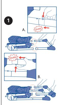
The ends of the front and rear legs have a different shape to avoid errors in the assembly phase.
