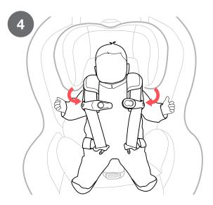
Adjust Harness Strap height position up or down by squeezing Adjustment Handle on top of Head Rest. Make sure Head Rest locks into position before tightening Harness.
