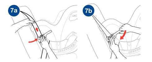
Unzip seat padding (a). Pull seat padding to the side and route vehicle lap belt through the blue REAR-FACING seat belt path on the side of Child Restraint (b).
