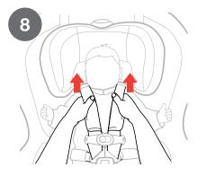
Tighten the harness by pulling slowly on Harness Adjustment Strap until the harness is snug on child (a). If you can pinch a fold in the strap at the child's shoulders, harness is too loose (b). If the harness is too loose pull the Harness Adjuster strap more.
