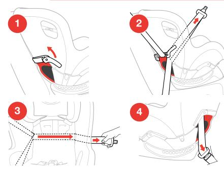
While pushing down on the Child Restraint (a) pull the vehicle shoulder belt (b) to tighten vehicle lap belt.
