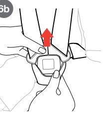
Fasten Chest Clip by snapping both sides together; listen for a click. Press the button on the Chest Clip and slide into desired position.
