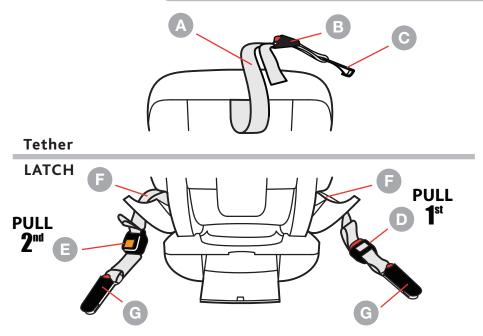
Always make sure LATCH Components are properly stored in the compartments when not in use.
