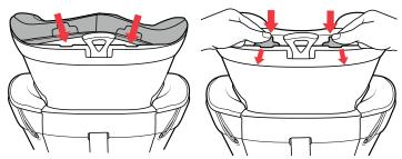
Tuck the fabric into the groove at the top of the headrest. Push down gently on both of the plastic tabs at the top of the Headrest until they snap into the grooves.
