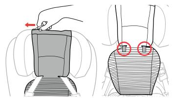
**Re-attach the Seat Back Air Mesh pad** by zipping the pad at the top of the headrest. Then attach both hook and loop tabs to the underside of the Headrest fabric below the Air Mesh pad.
