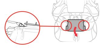
Diff up on the Latch Storage Compartment door, wrap both elastic straps on the Seat Bottom Pad around each end of the Latch Storage Compartment door, as shown. Close the Compartment door.
