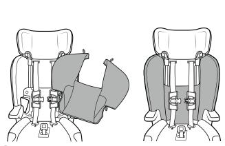
• Place the Backrest Seat Pad onto the Child Restraint.
