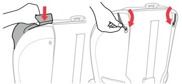
Tuck the fabric into the groove gently around the Child Restraint. Repeat for the other side. Hook BOTH elastic straps onto the back of the Child Restraint.
