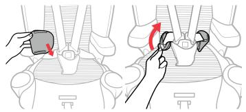
To attach the both Waist Belt pads, wrap one of the pads around the Harness Waist Strap and attach the hook and loop fasteners, repeat for the other Waist Belt pad.
