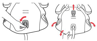
Place the Seat Bottom Fabric onto the Child Restraint and pull fabric around the Harness Adjuster Strap Cover. Then pull the Crotch Strap UP through the fabric and pull the FABRIC down and around the front and sides of the seat.
