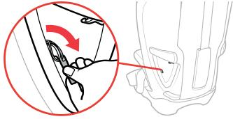
**S** Hook the Armrest fabric loop onto the side hook located near the vehicle belt path. Repeat this step for the other side. TIP: To Assist in the attachment of the Armrest fabric, push back on the fabric while hooking the loop.
