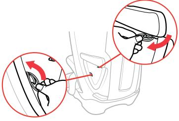
Unhook the elastic strap from the side hook and the top hook located near the vehicle belt path. Repeat for the other side.
