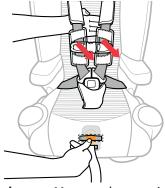
① Completely loosen Harness by pressing Harness Release Button on the front of the Child Restraint and pulling out on both of the Harness Straps. Then unbuckle the Chest Clip and Harness Buckle.
