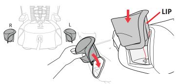
Match the "R" and "L" Cup Holders to the Child Restraint, and insert the Cup Holder. Make sure the Lip fits behind the groove and it clicks into place. Repeat this step for the other Cup Holder.
