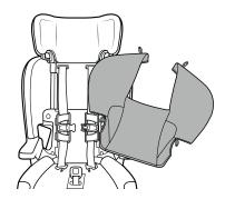
**W** Remove the Backrest Seat Pad from the Child Restraint.
