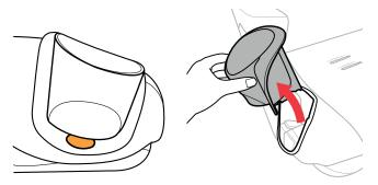
Remove BOTH of the cup holders by pressing the orange button located on the bottom edge of the Cup Holder and lifting up.
