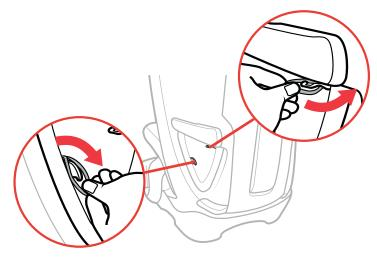
2 Hook the elastic strap onto the side hook and the top hook located near the vehicle belt path. Repeat for the other side.
