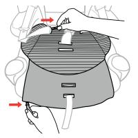
Remove the Seat Bottom Air Mesh pad by unzipping the pad at the back and front of the seat bottom. Thread the Crotch Strap down through the fabric and remove the Air Mesh Pad.
