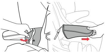
Undo the snap attaching the Armrest Fabric to the Backrest Seat Pad and then remove the Armrest Fabric. Repeat this step for the other Armrest.
