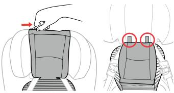
Semove the Seat Back Air Mesh pad by unzipping the pad at the top of the headrest. Then unhook both hook and loop tabs near the Shoulder Belt Guides.
