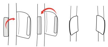
(5) Re-attach Shoulder Pad by folding the hook and loop Tab over the Harness Strap. Secure both hook and loop sides together. Repeat for the other Shoulder Pad and make sure they are oriented, as shown.
