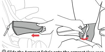
• Slide the Armrest Fabric onto the armrest then snap the Armrest Fabric to the Backrest Seat Pad. Repeat this step for the other Armrest.
