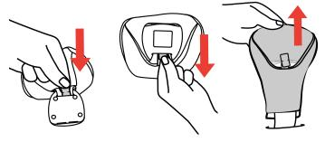
4 Remove the Crotch Strap Pad by pushing the fabric Tab through the slot on the BACK of the Harness Buckle. Then pull the Tab out of the FRONT and remove Crotch Strap Pad.
