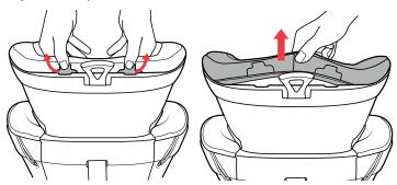
11 Pull back gently on both of the plastic tabs at the top of the Headrest and pull up on the Headrest fabric.
