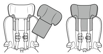
6 Place the Headrest Fabric Pad onto the Headrest.
