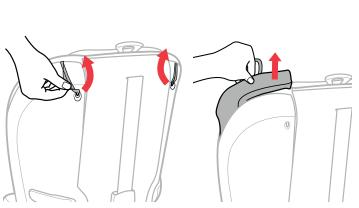
Unhook BOTH elastic straps on the back of the Child Restraint. Pull the fabric out gently from the groove around the Child Restraint. Repeat for the other side.
