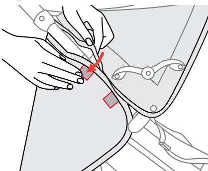
19. Attach the back panel of the canopy to the front of the canopy using the hook and loop fasteners on both sides.
