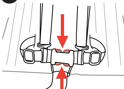
9. To open harness, release the waist clips from the center buckle as shown.
