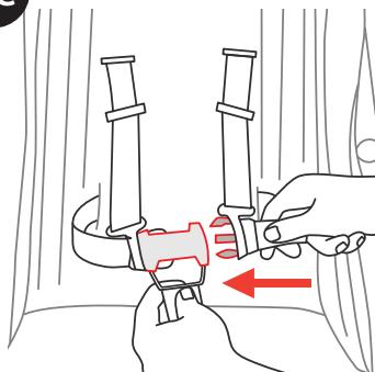
7. After sitting your child in the stroller, fasten the safety harness, first inserting the two prongs into the hole located on the shoulder straps (fig. 7A and 7B) and then into the buckle of the crotch strap (fig. 7C). Adjust the length of the straps to fit the child's shoulders and body correctly. To unfasten the waist strap, press and pull the side prongs.
