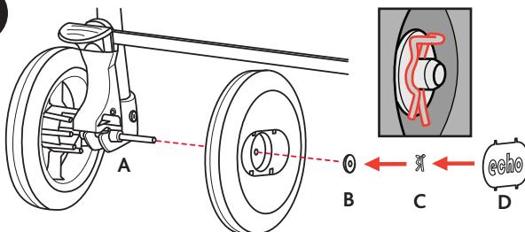
5. To assemble the rear wheels, insert the pin with the flat end (A) through a wheel and into the hole at the end of the rear leg tube assembly. Then insert another wheel onto the pin on other side as shown. Fit a washer (B) onto the pin and insert the clip (C) through the pin to secure both wheels. Finish off the assembly by attaching two wheel covers (D) on both wheels. Repeat this step for other rear wheel assembly.
