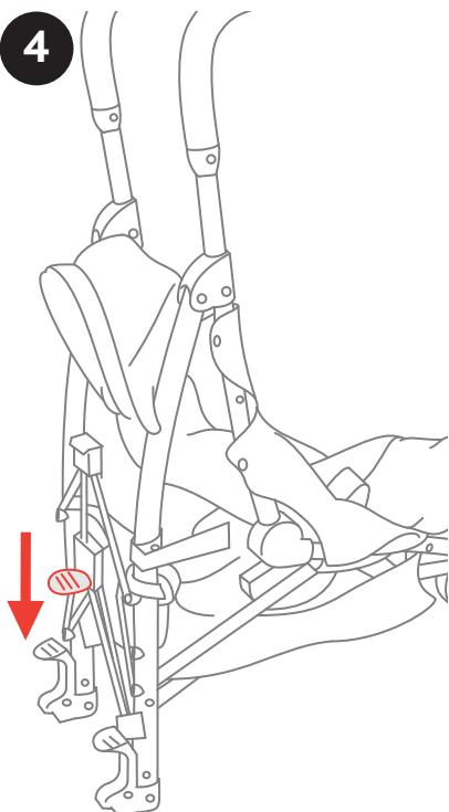
4. Push the rear locking mechanism downward with your foot.
