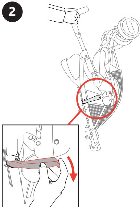
2. Hold the stroller by the handles in a vertical position, with the wheels facing forward. Release the closing device as shown.
