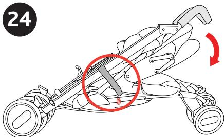
24. The stroller has an automatic locking system. Close the stroller ensuring that the closing device located on the side of the stroller is locked correctly. This operation prevents the accidental opening of the stroller.
