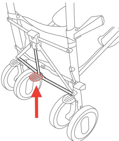
21. To close the stroller, first fold the canopy following the instructions shown in diagram 18. Pull the Rear Locking mechanism in an upward direction.
