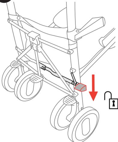
22. Release the secondary lock, by pressing the pedal on the right side of the stroller's frame with your foot.
