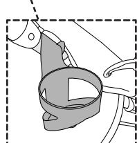
16. Attach the cup holder to the middle of either rear leg tube by clipping the lower portion first, then gently pressing the top portion to snap over stroller tube. It will help to gently flex the plastic to open up the clip. Remove cup holder by gently pulling the top portion first then un-clip the lower portion to release.
