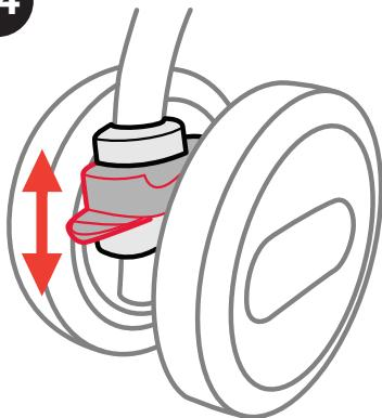
14. Use the swivel wheels on smooth surfaces. To lock the swivel wheels, raise the lever located between the two wheels. To unlock the wheels, push the lever in a downward direction.
