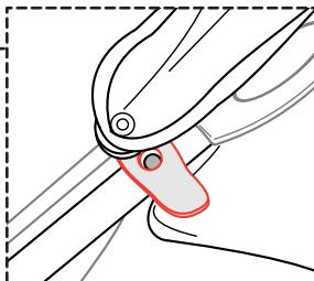
17. To fit the Canopy, fasten the canopy clip to stroller frame as shown. Be sure the **button on the frame** nests into the hole on the canopy clip. Make sure both sides of the Canopy are clipped to the frame as shown.
