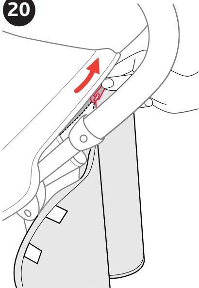
20. The Canopy can become a Summer Canopy by removing the rear panel. Unzip the rear panel from the canopy near the stroller handles. Then undo the hook and loop fasteners at the sides of the canopy.
