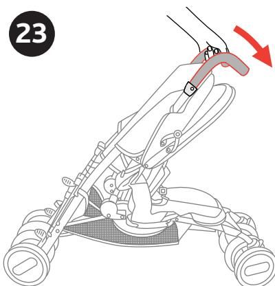
23. To close the stroller completely, push the handles forward.
