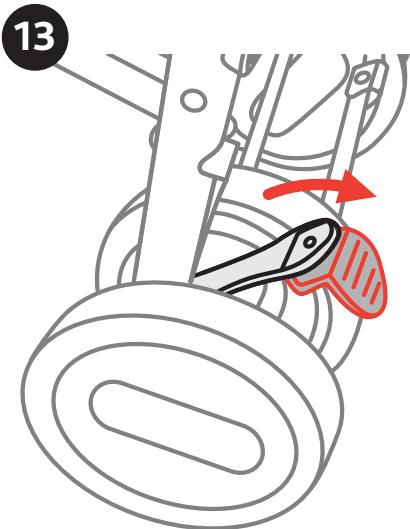
13. To apply the brakes, push on both of the two levers located at the centre of the rear wheels in a downward direction. Reverse direction to unlock the brakes.
