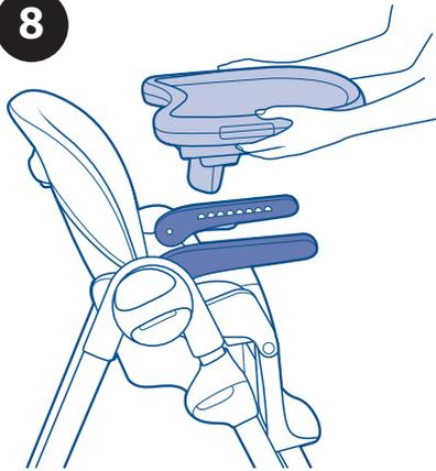
8. The tray can now be fitted to the Highchair. Line up the tray guides with armrests and push down on tray.
