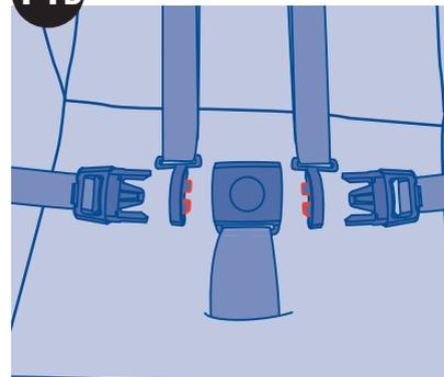
14B. The Highchair has a 5-point safety harness. The Shoulder Strap Connector is designed to break away from the Waist Clip when not secured in the Crotch Strap Buckle.
