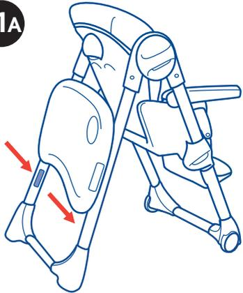
11. When not in use, the tray can be stored on the rear legs of the frame by using the rear leg slots as shown in 11A. With the tray resting against the rear legs, above the slots and locking guides on the inside of the rear legs, allow the tray to slide down the legs and lock into rear leg slots (diagram 11B). To release the tray press the locking button and remove from the legs.
