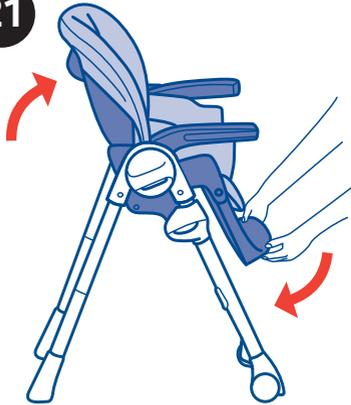
21. Place the backrest in a upright position, and rotate the footrest down.
