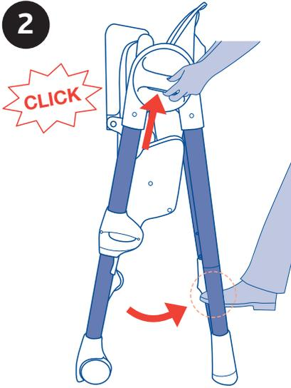
2. Stand at the back of the highchair and hold the two side joints, then press the open/close buttons. At the same time, open the Highchair legs using your foot, until an audible click is heard, signalling that the legs are locked in the open position (diagram 2).
