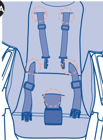
14A. Fit the Highchair cover to the Highchair seat. Thread the shoulder straps, waist belt and crotch strap through the corresponding openings (diagram 14A). Make sure the shoulder straps are at the appropriate height position and the waist belt is pulled through the seat fabric. Repeat steps 14A, 14B, 14C and 14D with second cover (included only on certain models).
