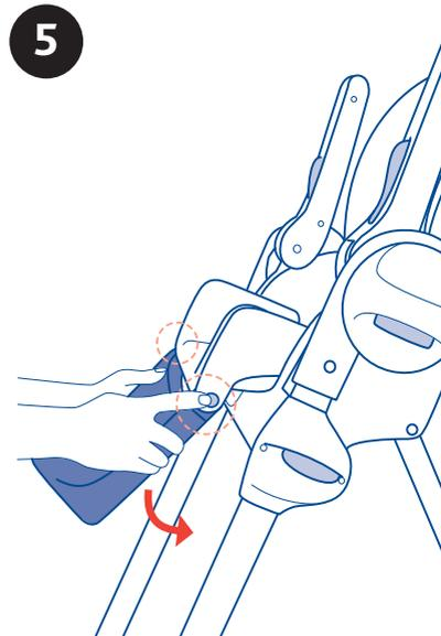
5. Press the side adjustment buttons and lower the leg rest in a vertical position (diagram 5).
