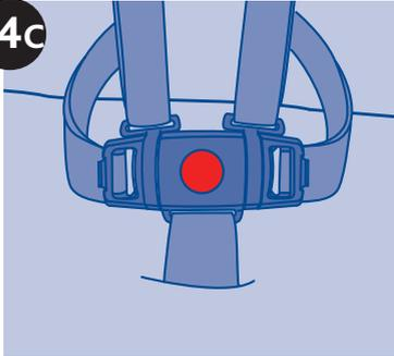
14C. The safety harness can be released by pressing the button on the center of the Crotch Strap Buckle and pulling both Waist Clips out.
