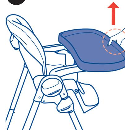
10. To remove the tray, you must squeeze the release button under the tray, then pull up or off.
