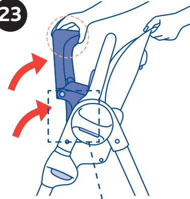
23. Lift up on seat pad and locate the back edge of the seat. Unsnap the seat from the frame. Fold up the seat and leg rest as shown.
