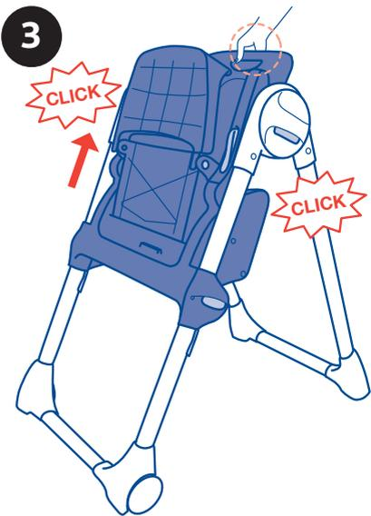
3. Raise the seat by holding the upper part of the backrest and pull it upward, until the desired height is reached (diagram 3). The Highchair can be adjusted to 7 height positions.
