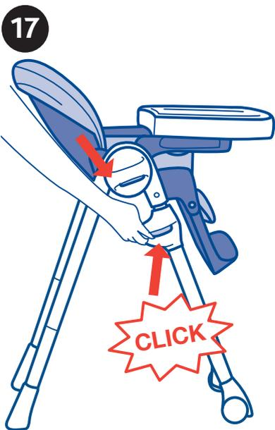
17. To lower the seat: Press the two side buttons simultaneously and lower the seat, until the desired height is reached (diagram 17).
