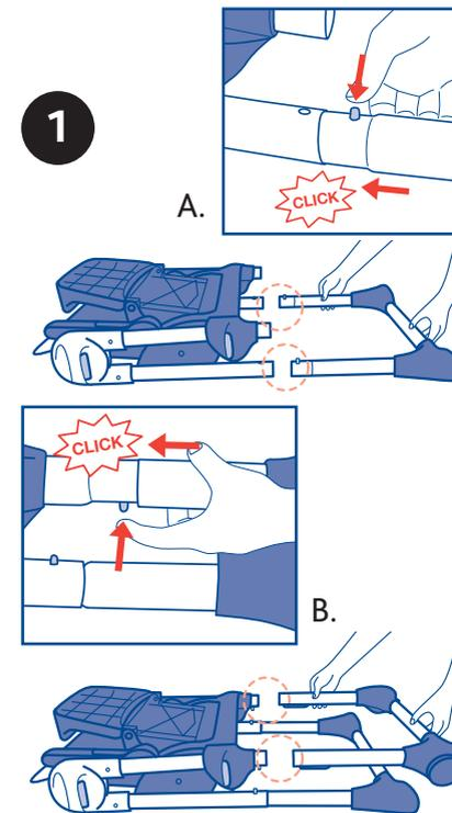
The ends of the front and rear legs have a different shape to avoid errors in the assembly phase.
