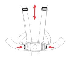
The length of the Shoulder Straps can be adjusted by pulling on the adjustment buckles to tighten or loosen. The length of the waist straps can be adjusted. Press the tab at the end of the Waist Strap Clip and pull on the strap to tighten or loosen, to better fit your child.
