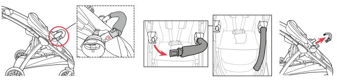
To remove Armbar, press in on the buttons located at the sides of the Armbar, as shown. Undo one side of the Armbar, and swing away to the side. Undo both sides and remove completely. To re-attach the Armbar insert the Armbar Tongues into the corresponding openings on the Seat Frame.
