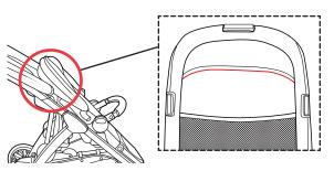
**To adjust the Shoulder Harness to another height position,** locate the D-ring on the back of the seat as shown.
