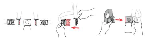
This stroller has a 5-point safety harness. The Shoulder Strap Connector is designed to break away from the Waist Clip when not secured in the Crotch Strap Buckle. Make sure the Shoulder Strap Connector is in the correct position, as shown. Slide the Shoulder Strap Connector onto the Waist Strap Clip and repeat for the other side. Then slide both Waist Clips into the Crotch Strap Buckle, as shown. Pull on both sides to make sure the Clips are secured to the Buckle.
