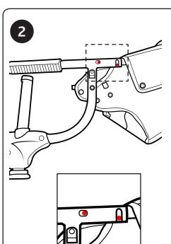
2. When the arm is on as far as it will go, twist it until the buttons on the side piece click into place in the holes of the arm. Repeat these steps with the arm on the other side of the chair.
