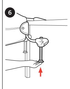
6. Push the pin on one arm up until it is resting firmly against the bottom of the table. It will click as it moves through each possible position. Repeat this step with the pin on the other arm.
