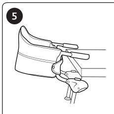
5. Hold the chair in position on the table so that the arms are level with the table surface. Push the chair onto the table until it cannot go any further. Check to make sure there is not a gap between the edge of the table top and the arms.
