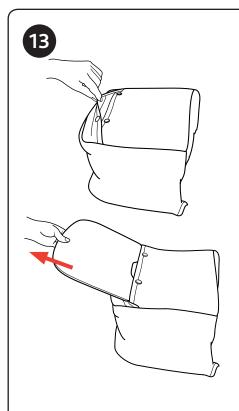
13. Release the snaps on the bottom of the seat and remove the rigid base.
