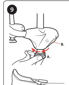
9A. Unlock the pins by turning the screws on the end of the pins in a clockwise direction.
