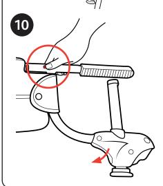
10. To fold the chair, press the front button on each side of the chair and fold the arms toward the center of the chair.
