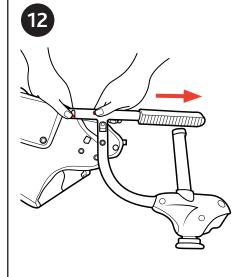
12. Press the buttons on both side pieces and slide the arms over the buttons and off of the chair. At this point, you can remove the fabric from the seat frame.
