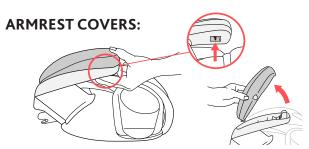
• Locate the Armrest release button directly under the front of the Armrest. Pull on the button and at the same time lift up on the front edge to remove the Armrest pad.
