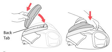
• **To reattach the Armrest**, insert the Back Tab into the Armrest base and push down on the front edge until it clicks into the base.
