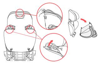
**Lift up on the plastic tabs** at the top of the Headrest and below the Shoulder Belt Guides, as shown. Pull the Seat fabric cover forward to remove.
