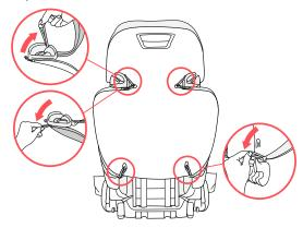
On the Booster Backrest, unhook 6 elastic loops as shown. Four behind the Headrest and two at the bottom of the seat back.
