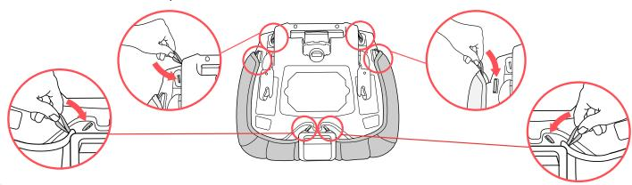
Position the fabric cover on the Booster Seat bottom and tuck in the fabric along the belt guide edges. Flip the seat bottom over. Then tighten the fabric over the Booster Seat bottom further by reattaching the elastic loops, as shown.
