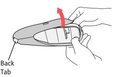
**Pull back on the edges** of the Armrest fabric covers and slide the fabric off the Armrest base.
