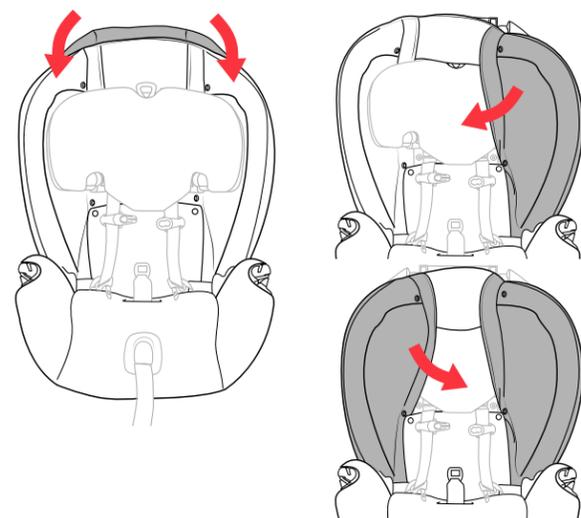
22 With the Child Restraint facing you, pull forward on the fabric. Guide it off of the Child Restraint Seat frame and then around the Headrest frame.
