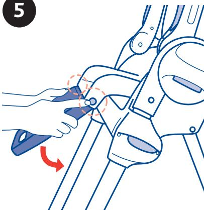
5. Press the side adjustment buttons and lower the leg rest in a vertical position (diagram 5).
