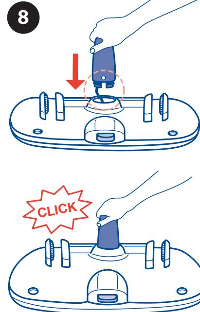
8. Insert the Crotch Bar into the cooresponding opening on the tray. Make sure the tether does not hinder the Crotch Bar from snapping into place. The design of the Crotch Bar allows it to only be assembled one way.
