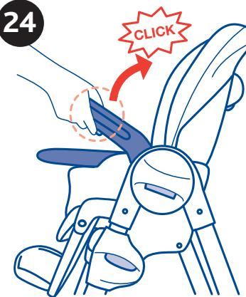
24. Raise the armrest in a vertical direction by pressing the buttons located on the lower part of the arm rests, until an audible click is heard (diagram 24).
