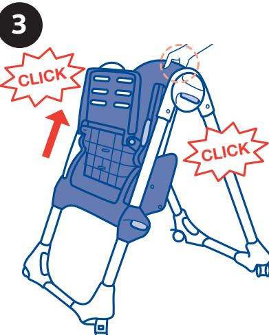
3. Raise the seat by holding the upper part of the backrest and pull it upward, until the desired height is reached (diagram 3). The Highchair can be adjusted to 7 height positions.
