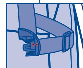
15B. Attach the shoulder harness to the waist belt clip. Hold the waist belt clip stationary and line up the arrows on the shoulder harness clip and waist belt clip. Push the shoulder harness clip down into the waist belt clip (twisting motion), it will click into place.
