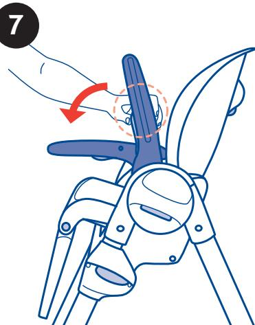
7. Lower the armrests by pressing the two buttons located at the bottom of the armrests (diagram 7).
