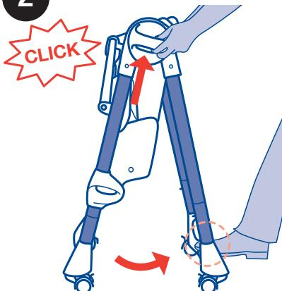
2. Stand at the back of the highchair and hold the two side joints, then press the open/close buttons. At the same time, open the Highchair legs using your foot, until an audible click is heard, signalling that the legs are locked in the open position (diagram 2).
