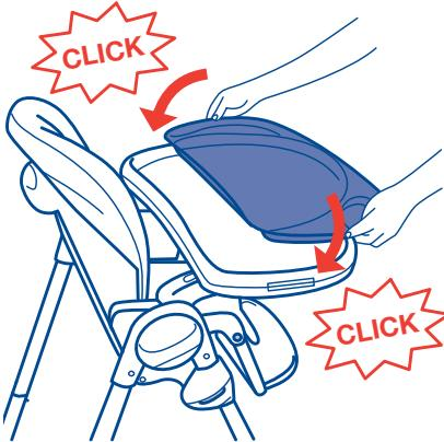
13. The Highchair has a tray cover. This can be attached by firmly pushing down on the outside area of the tray until it clicks into place, as shown. To remove the tray pull out on the outside edge of the tray and lift up.
