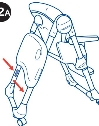
12. When not in use, the tray can be stored on the rear legs of the frame by using the rear leg slots as shown in 12A. With the tray resting against the rear legs, above the slots and locking guides on the inside of the rear legs. Allow the tray to slide down the legs and lock into rear leg slots (diagram 12B). To release the tray press the locking button and remove from the legs.
