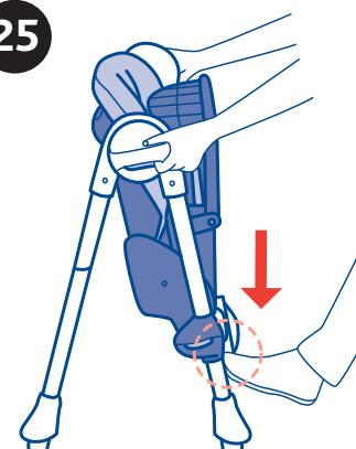
25. Lower the seat by pressing the two side buttons at the same time, as shown in the diagram 25.
