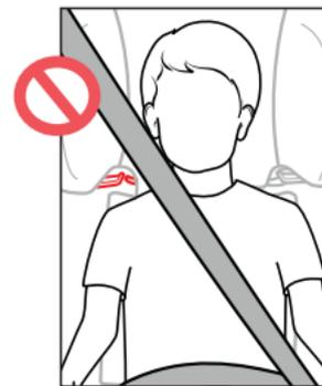
⚠ To avoid injury to others, ALWAYS secure this child restraint in BOOSTER MODE when unoccupied. An unsecured Booster Seat could injure other occupants in a sudden stop or crash.
