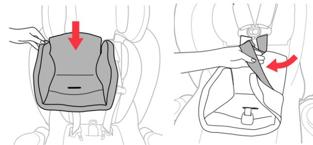
**27 Place the Stage 1 Positioner on the Child Restraint.** Thread the Shoulder Straps into the side openings on the positioner pad and thread the Harness Buckle up into the correct slot in the pad.
