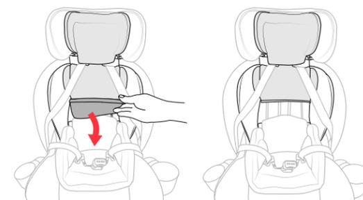
**29 Before lowering the Headrest to the lowest position,** lift up on the bottom edge of the Headrest Insert. Locate the lower portion of the Headrest Pad and fold it under.
