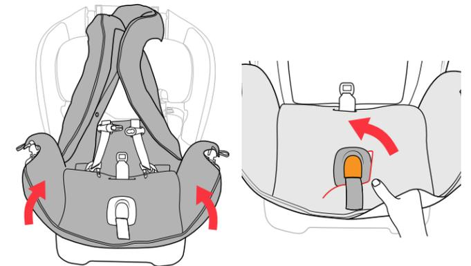
25 **Thread the Harness Buckle down** through the slot in the pad and pull the **FABRIC** up around the front and sides of the seat frame. Then carefully pull fabric around the Harness Adjuster Strap Cover and remove the Seat Bottom Pad. The plastic Harness Adjuster Strap Cover is **NOT** removable. Remove the Fabric.
