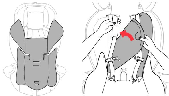
**20 Place the Stage 2 Positioner on the Child Restraint.** Thread the Harness Buckle up through the correct slot in the seat pad and pull the Shoulder Straps over the Stage 2 Positioner and into the side openings in the seat pad.
