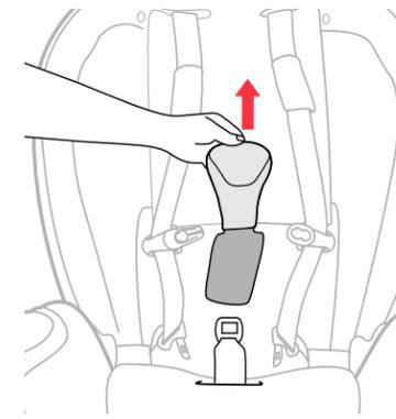
**14 If desired, attach the Crotch Strap Pad for Stage 3 & 4 use.** Thread the Crotch Strap Pad tongue down into the same opening as the Harness Buckle (See Step 5 and 6 in Softgoods Removal Stage 1).
