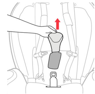
**26 Remove the Crotch Strap Pad** by pulling the Crotch Strap Pad up and off the Harness Buckle, as shown. Lower the Headrest to the lowest position.
