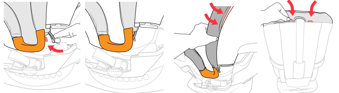
8 Locate the elastic strap near the back of the Lap Belt Guide, pull on the strap and tuck the fabric around the upper edge of the Lap Belt Guide. Wrap the elastic strap around the post inside the LATCH belt compartment. Close the compartment and repeat for the other side.
