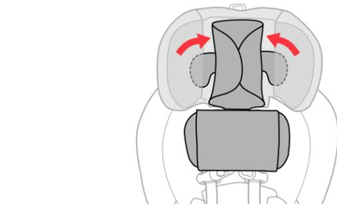
10 **Slide both Headrest Flaps** from the side pockets on the Headrest. Remove the Stage 1 & 2 Headrest Insert from the Child Restraint.
