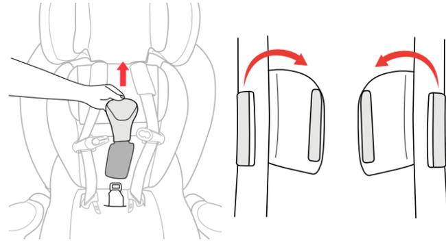
8 **Remove the Crotch Strap Pad** by pulling the Crotch Strap Pad up and off the Harness Buckle, as shown. Also remove the Shoulder Pads, if desired.
