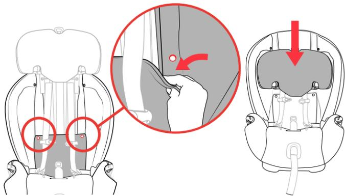
20 **Undo both snap buttons on the inside of the seat pad**, as shown. Then lower the Headrest to the lowest position.
