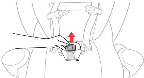
**5** If desired, Reattach the Crotch Strap Pad and Shoulder Pads for Stage 2 use. Pull the Harness Buckle forward and insert the Crotch Strap Pad tongue down into the same opening as the Harness Buckle. The Crotch Strap Pad tongue will be behind the Harness Buckle. Thread the Harness Buckle up into the Crotch Strap Pad.
