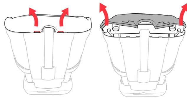
21 **At the top edge of the seat back**, pull back gently on both of the plastic tabs and lift up fabric. Remove the fabric from the top edge of the seat back.
