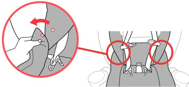
12 **Locate and undo both side snap buttons,** as shown.
