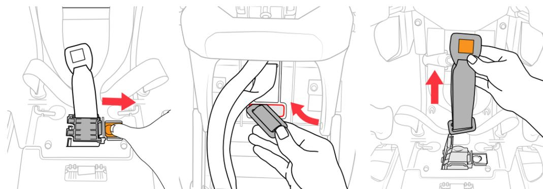
26 **Open the Crotch Strap Lock and fully recline the seat (Position 1)**. Tilt the Child Restraint back and locate the crotch strap metal bar underneath the seat. Turn metal bar slightly and push the corner through the slot. Work the metal bar through the slot while pulling Harness Buckle out on the other side.
