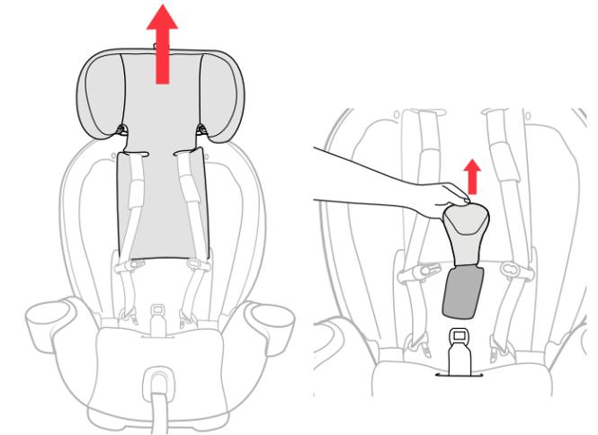
**17 Raise the headrest to the highest position** and remove Crotch Strap Pad.
