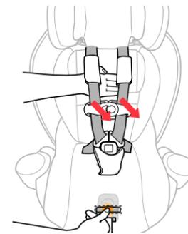
**25 Completely loosen Harness** by pressing Harness Release Button on the front of the Child Restraint and pulling out on both of the Harness Straps. Then unbuckle the Chest Clip and Harness Buckle.
