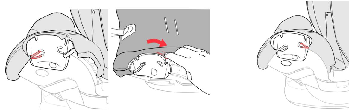
4 While pulling on the Front elastic strap, press in on the fabric guiding it into the groove. Wrap the elastic strap around the post inside the Cup Holder cutout. Tuck the fabric edge around the outside Cup Holder frame, making sure the grooves in the Cup Holder frame are not covered by the fabric.
