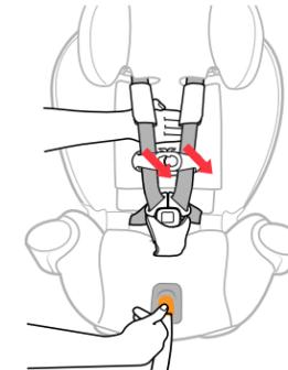
15 **Completely loosen Harness** by pressing Harness Release Button on the front of the Child Restraint and pulling out on both of the Harness Straps. Then unbuckle the Chest Clip and Harness Buckle.
