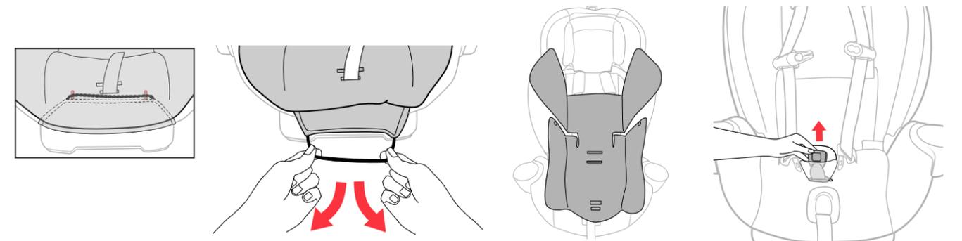
14 **Unhook the elastic loop below the front edge of the Child Restraint,** and thread the Harness Buckle down through the slot in the pad. Remove the Stage 2 Positioner from the Child Restraint. If desired, re-attach the Crotch Strap Pad and Shoulder Pads for Stage 3 use. Thread the Crotch Strap Pad tongue down into the same opening as the Harness Buckle (See Step 5 and 6 in Softgoods Removal Stage 1).
