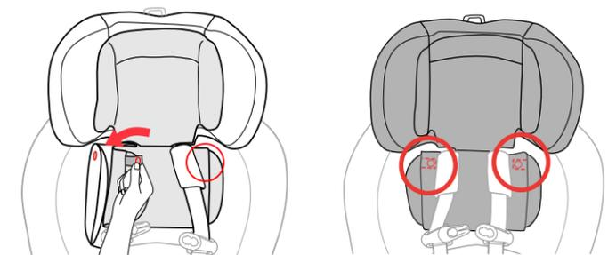
**19 Slide Shoulder Straps into Headrest Slots, then attach both snap buttons located on the bottom section of the Stage 1 & 2 Headrest Insert, as shown.**
