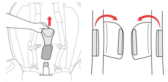
16 **Remove the Crotch Strap Pad** by pulling the Crotch Strap Pad up and off the Harness Buckle, as shown. Also remove the Shoulder Pads.
