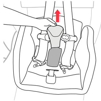
**2** Remove the Crotch Strap Pad by pulling the Crotch Strap Pad up and off the Harness Buckle, as shown.
