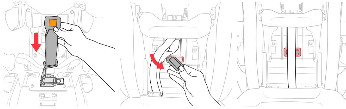
27 Guide one corner of the metal bar through slot in the Crotch Strap Lock compartment. With the seat fully reclined (Position 1), pull the metal bar through the slot from underneath the seat. Make sure the metal bar lays flat on the bottom of the seat, as shown.
