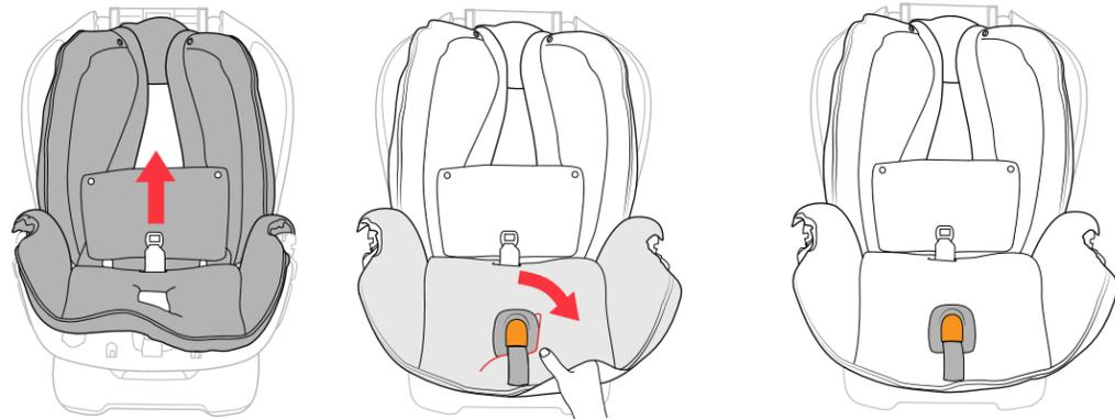
1 Make sure the Headrest is in the lowest position and open the LATCH storage compartments. Place the Seat Pad onto the Child Restraint frame and thread the Harness Buckle up through the correct slot in the seat pad. Then carefully guide the fabric around the Harness Adjuster Strap Cover.
