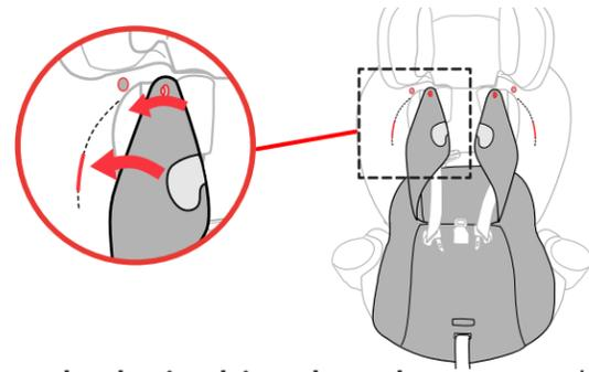
**21 Insert the plastic tab into the pocket crease,** and attach the top snap button on the Stage 2 Positioner side wing. Repeat for the other side. Double check to make sure the plastic tab is pushed all of the way down into the pocket.
