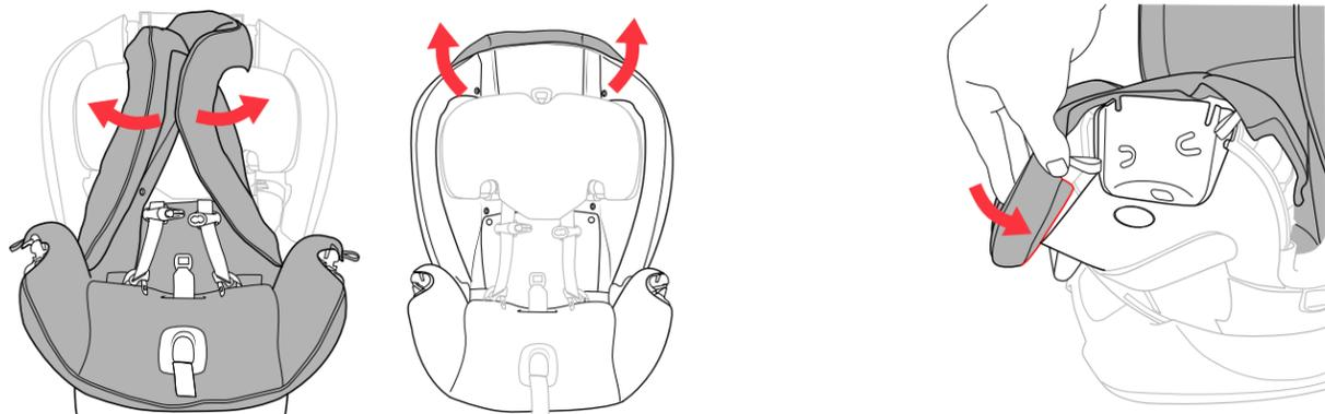
2 Pull the fabric down and around the front edge and insert the headrest into the top opening in the fabric. Pull the fabric around the back of the Seat Frame.
