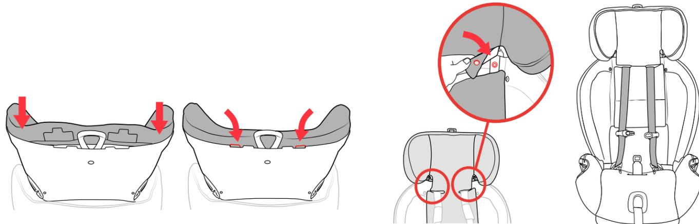
**11 At the back edge of the Headrest** locate the plastic tabs. Press them into the headrest frame until they click into position, as shown.
