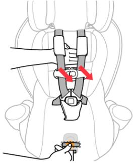
7 **Completely loosen Harness** by pressing Harness Release Button on the front of the Child Restraint and pulling out on both of the Harness Straps. Then unbuckle the Chest Clip and Harness Buckle.
