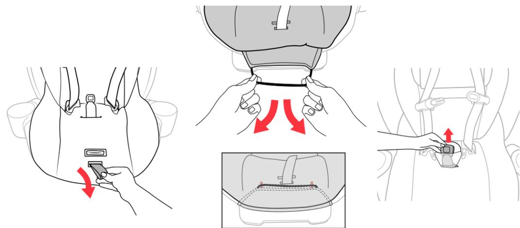
**24 Locate and pull the adjuster strap through the opening on the seat pad.** Attach the elastic strap on the front of the Stage 2 Positioner by pulling the elastic strap under the front edge of the seat bottom and loop it around both hooks. If desired, re-attach the Crotch Strap Pad for Stage 2 use.
