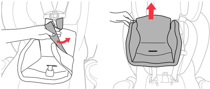
**3** Remove the Stage 1 Positioner by pulling the Shoulder Straps out through the side openings on the pad and thread the Harness Buckle through the slot in the pad. Remove the Stage 1 Positioner from the Child Restraint.
