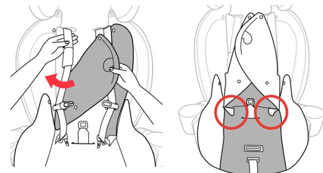
13 **Thread the Shoulder Straps out through the side openings** on the Stage 2 Positioner. Pull forward on the seat fabric and Stage 2 Positioner, as shown. Then reach under the seat bottom fabric and undo both Snap Buttons attaching the Stage 2 Positioner to the seat bottom fabric.
