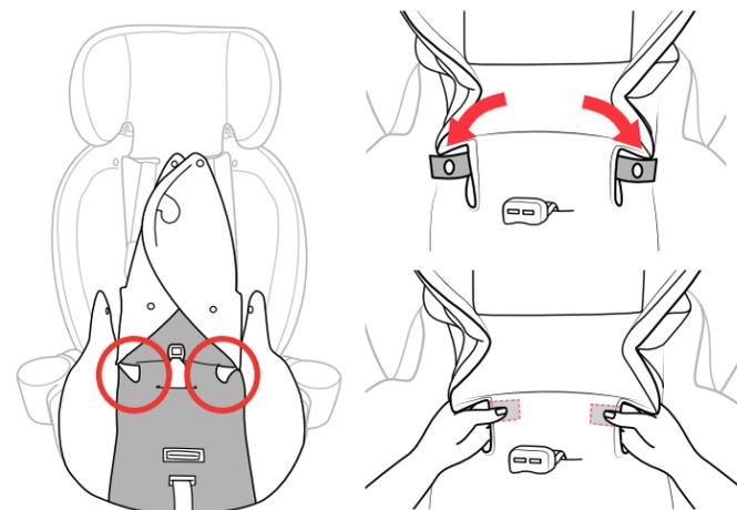
**23 Pull forward on the seat fabric and Stage 2 Positioner,** as shown. Wrap both snap button straps down and under the seat fabric. Using your fingers, line up and attach both snap buttons to the underside of the seat fabric.
