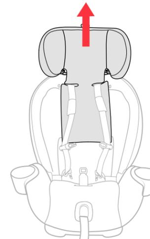
17 **Raise the headrest to the highest position** and remove BOTH of the Cup Holders. Press the orange button located on the bottom edge of the Cup Holder and lift up, repeat for the other side.
