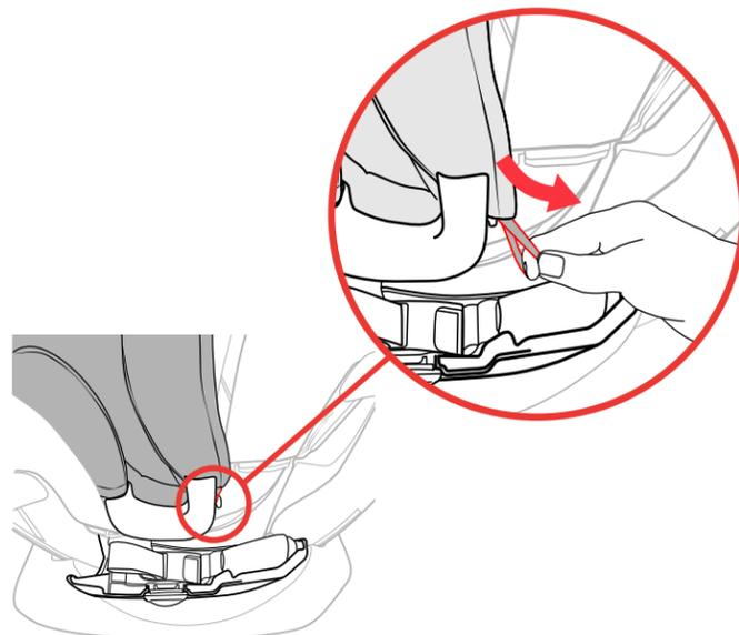
23 **On one side of the Child Restraint open the LATCH Storage compartment**. Locate and unhook the elastic loop, as shown. Pull the fabric edge out and around the orange Lap Belt guide.
