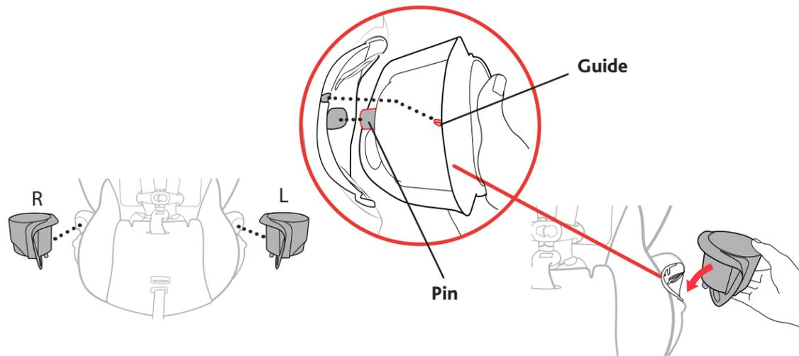
**13 Attach the Cup holders to the Child Restraint.** Match the "R" and "L" Cup Holders to the Child Restraint, as shown. Make sure the fabric is tucked in along the Child Restraint lip to allow the Cup Holder to be attached properly. Line up the Cup Holder pin and the two guides with the openings on the Child Restraint, as shown. Push in and then push down on the Cup Holder until it clicks into place. Repeat for the other side.
