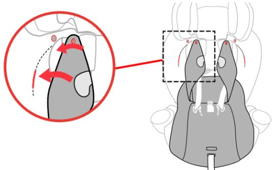
11 **Locate and undo the top snap button on the Stage 2 Positioner side wing.** Below the snap button, pull the plastic tab from the pocket. Repeat for the other side.
