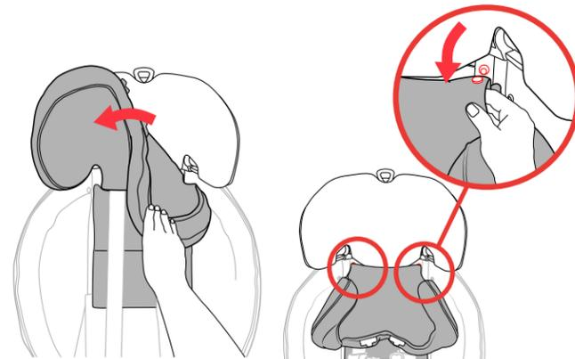
19 **With the Child Restraint facing you**, pull forward on the fabric and guide it off of the Headrest frame. Undo both snap buttons holding the headrest fabric in place at the bottom of the Headrest frame, as shown.
