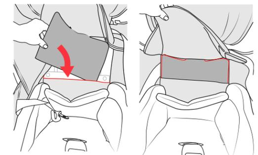
**30 Tuck the bottom Headrest Pad** behind the Stage 2 Positioner pad, but in front of the Stage 3 & 4 seat pad, as shown.
