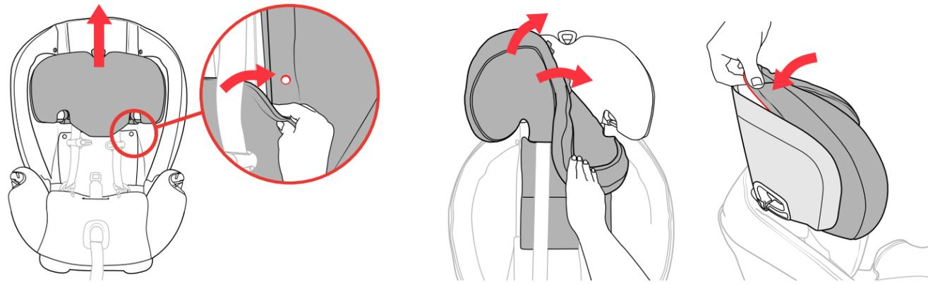
**10 Attach both snap buttons on the seat fabric, as shown.** Pull the Headrest up to the highest position. Slide the Headrest fabric onto and around both sides of the Headrest frame. Tuck the fabric edges into the Headrest frame edges, as shown.
