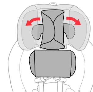
**18 Slide both Headrest Flaps** into the side pockets on the Headrest.
