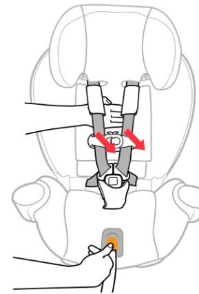
**16 Completely loosen Harness** by pressing Harness Release Button on the front of the Child Restraint and pulling out on both of the Harness Straps. Then unbuckle the Chest Clip and Harness Buckle.
