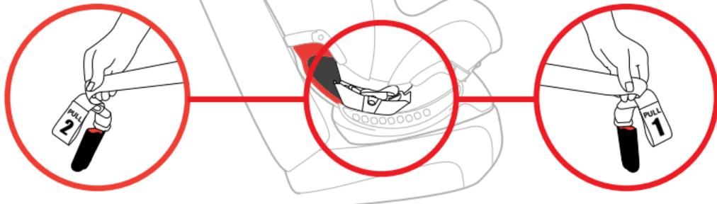
Make sure LATCH Adjuster strap (Pull 1<sup>st</sup>) is loosened to the full length.
