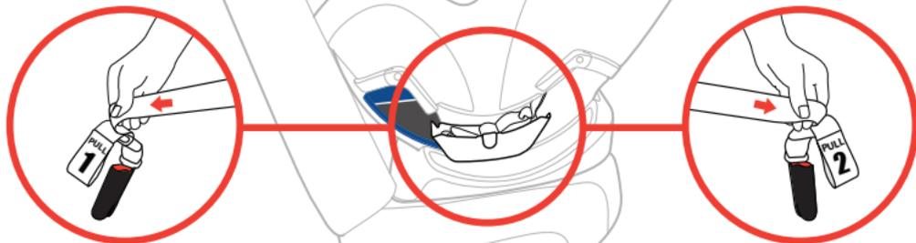
Make sure SuperCinch™ LATCH Tightener strap (Pull 2<sup>nd</sup>) is loosened to the full length.
