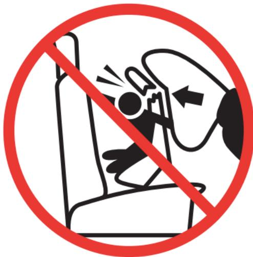
**⚠ WARNING! WHEN USING THIS CHILD RESTRAINT REAR-FACING, DO NOT PLACE THIS CHILD RESTRAINT IN A VEHICLE SEATING LOCATION WITH A FRONTAL AIR BAG, UNLESS THE AIR BAG CAN BE TURNED OFF.**
