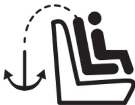
Tether anchor locations vary from vehicle to vehicle. Check your vehicle owner's manual and look for the tether anchor symbol as shown. A tether reduces movement of a forward facing child restraint in a crash and helps to achieve a tight installation.
