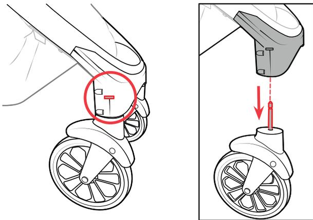
1 Remove the Front Wheels by **pushing in on the Release Button, just above the wheel** (as shown). And, at the same time, pull the Front Wheel off of the Stroller Frame. Repeat for the other Front Wheel.
