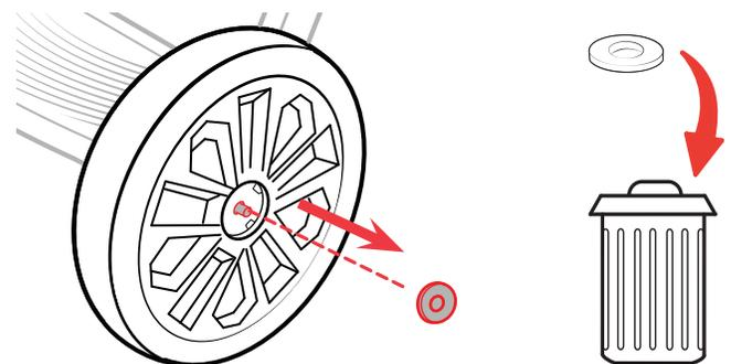
4 Remove the Washer from the Rear Axle. **Discard the old Washer.**
