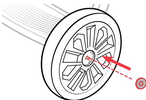
7 On the same side, **slide a Washer onto the Rear Axle.**
