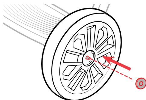
7 On the same side, **slide a Washer onto the Rear Axle.**
