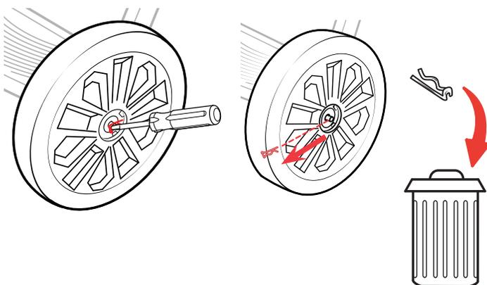
3 Remove the Pin from the Rear Axle using a flat blade screwdriver, as shown. **Discard the old Pin.**
