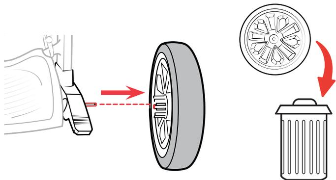
5 Remove the Wheel from the Rear Axle. **Discard the old Wheel. Repeat Steps 2-5 for other Rear Wheel.**
