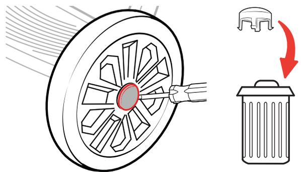
2 On one side of the stroller remove the Rear Wheel Hubcap using a flat blade screwdriver, as shown. **Discard the old Hubcap.**
