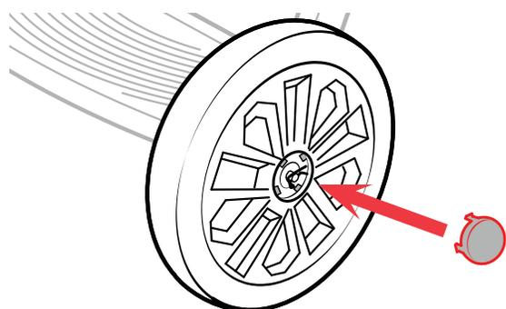
9 Line up the tabs on the Hubcap with the holes on the Wheel. **Snap the Hubcap onto the Wheel to cover the Washer and Pin. Repeat Steps 6-9 for other side.** Pull on each Wheel to make sure the Wheel assembly is securely attached to the frame.
