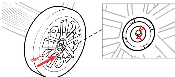
8 Secure the Wheel to the Rear Axle using the Pin. **Push the straight side of the Pin through the hole on the Rear Axle.** The curve on the Pin must curve around the outside of the Rear Axle, as shown. Make sure Washer is between the Pin and Wheel.
