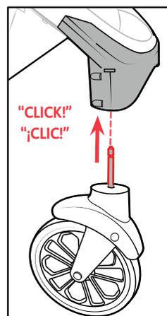
10 Attach the Front Wheel to the Stroller Frame, **line up and insert the Front Wheel Pin into the corresponding opening on the Stroller Front Leg, as shown.** Repeat for the other side.
