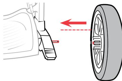
6 On one side of the Rear Axle, **slide on a Rear Wheel.** You may need to turn the Wheel until the brake tab fits into one of the grooves on the Wheel if the brake lever is down.
