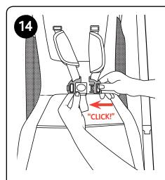
14. To secure your child, guide the child's arm through the waist belt and shoulder strap. Insert the waist belt clip into the crotch strap buckle. Repeat for the other side. Pull on both sides to make sure the Clips are secured to the Buckle.
