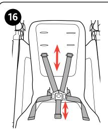
16. The length of the Shoulder Straps and Crotch Strap can be adjusted by pulling on the adjustment buckles to tighten or loosen.
