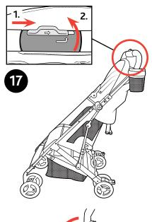
17. To fold the stroller, 1) slide the release button to the right. 2) Rotate the handle grip forward, at the same time push forward on the stroller handle.
