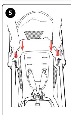
5. To attach the canopy (D), insert the canopy frame ends into the canopy mounts, as shown.
