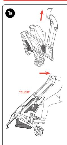
1B. At the same time, pull up on the stroller handle. Place your foot on the rear axle and pull back on the Stroller handle until the Stroller Frame clicks into place. Check to ensure that the Stroller Frame is locked in the open position.
