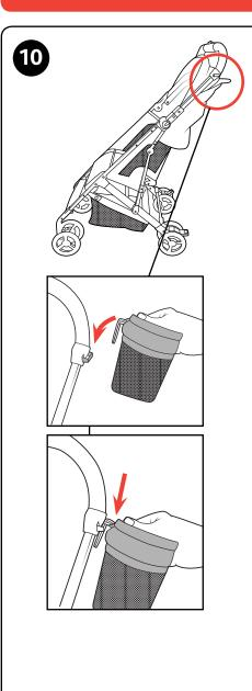
10. To attached the Cup Holder (C), locate the cup holder attachment on the Stroller Frame. Insert the Cup Holder wire hook into the cup holder attachment, as shown.
