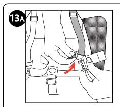
13A. To adjust the Shoulder Strap, slide the end of the strap through harness clip, remove the shoulder pad, and thread the strap through the opening on the seat back.
