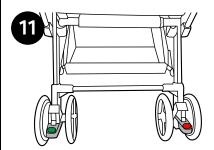
11. To engage the Stroller brakes, push down on the **RED** brake lever (11A) to lock the Rear Wheels. Pull back and forth to make sure that the brake is engaged. To unlock the Stroller, push down on the **GREEN** brake lever (11B) to unlock the Rear Wheels.
