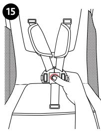
15. Unbuckle Safety Harness by pressing the button on the center of the crotch strap buckle. Pull out both waist belt clips.
