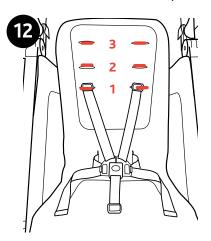
12. The Shoulder Straps can be adjusted to 3 height positions as shown.
