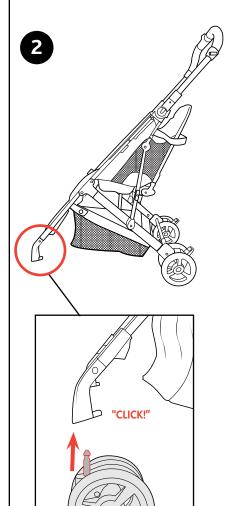
2. Attach the Front Wheel (B) to the Stroller Frame by lining up and inserting the Front Wheel Post into the opening on the frame, as shown. Repeat for the other side.
