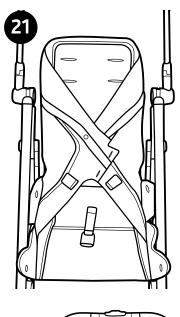
21. Unbuckle the harness straps and thread the shoulder straps through the back rest (refer to step 11). Pull up on the corner of the seat back and remove the seat fabric from the stroller frame, as shown.
