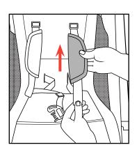
13B. Re-insert the Shoulder Strap into the correct opening on the seat back, and pull it through. Make sure the strap is not twisted. Re-attach the shoulder pad and thread the strap into the harness clip. Flatten the fabric tab against the harness clip. Pull on the shoulder strap to make sure it is securely attached to the harness clip. Repeat step 13 for the other side. Always use the same opening position for both shoulder straps.
