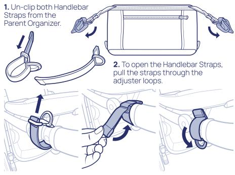
**3a.** Wrap one Strap around the Stroller Handle above the Handle Adjuster Button and push it up through the adjuster loop.
