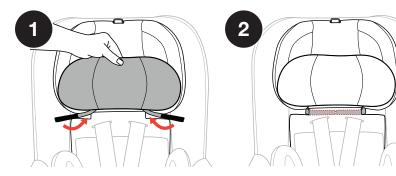
To Adjust Handle, press the Handle Release Button on one side and rotate the handle. There are 3 positions:
