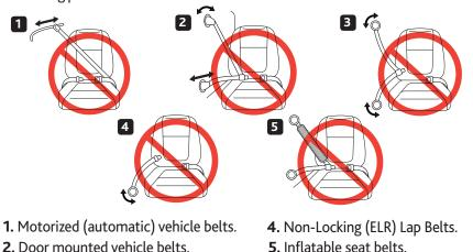
3. Lap-shoulder Belts with 2 retractors (unless Lap Belt has a "Lock Mode").
