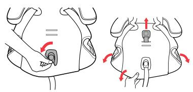
Place the Seat Bottom Fabric onto the Child Restraint and pull fabric around the Harness Adjuster Strap Cover.
