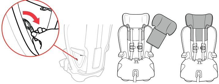
**Solution** Hook the Armrest fabric loop onto the side hook located near the vehicle belt path. Repeat this step for the other side. TIP: To Assist in the attachment of the Armrest fabric, push back on the fabric while hooking the loop.
