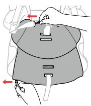
**Re-attach the Seat Bottom Pad,** thread the crotch strap through the correct opening in the pad. Then zip the pad at the back and front of the Seat Bottom Pad.
