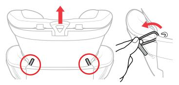
With the Headrest in the highest position, locate the elastic strap on the BACK of the Headrest and unhook by pulling up on the fabric tab. Repeat this step for the other elastic strap.
