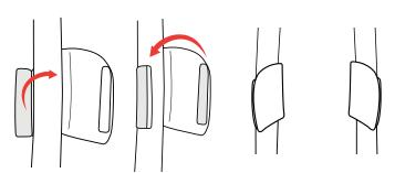
Tab over the Harness Strap. Secure both hook and loop sides together. Repeat for the other Shoulder Pad and make sure they are oriented, as shown.
