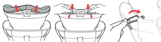
Tuck the fabric into the groove at the top of the headrest. Push down gently on both of the plastic tabs at the top of the Headrest until they snap into the grooves.
