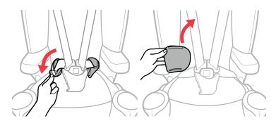
2 Undo the hook and loop fastener on BOTH Waist Belt pads and remove.
