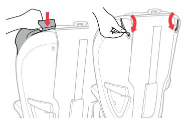
Tuck the fabric into the groove gently around the Child Restraint. Repeat for the other side. Hook BOTH elastic straps onto the back of the Child Restraint.
