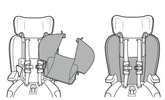
Place the Backrest Seat Pad onto the Child Restraint.
