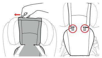
(3) Re-attach the Seat Back Pad by zipping the pad at the top of the headrest. Then attach both hook and loop tabs to the underside of the Headrest fabric below the pad.
