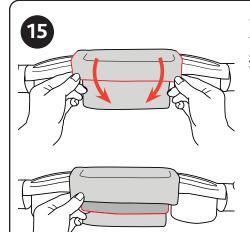
15. To remove the Accessory Pocket, flip out the plastic tab from the groove under the front of the Parent Tray.
