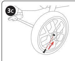
3C. Secure the Wheel to the Rear Axle using a Pin (F). Push the straight side of the Pin through the hole on the Rear Axle. The curve on the Pin must curve around the outside of the Rear Axle, as shown. Make sure Washer is between the Pin and Wheel. Repeat Steps 3A-3C for other side.
