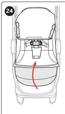
24. Lift up the Footrest Pad on the front of the stroller to locate two sets of straps. Both Straps have a Buckle under the Seat Pan. Reach under the Seat Pan and undo both Buckles.
