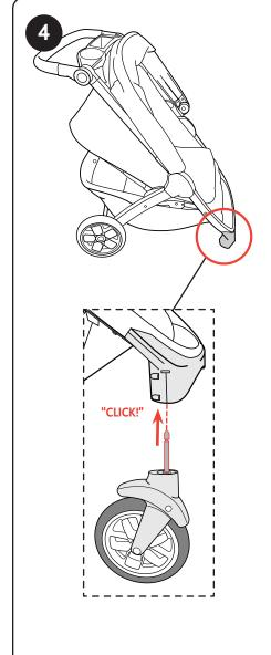
4. Attach the Front Wheel (B) to the Stroller Frame by lining up and inserting the Front Wheel Pin into the corresponding opening on the Stroller Front Leg, as shown. Repeat for the other side.
