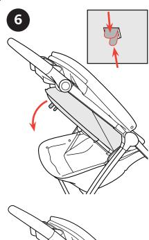
6. To Recline the Backrest, squeeze both levers together and pull down on the Backrest. To adjust the Backrest into an upright position, push up on the Backrest until it locks into the desired position.
