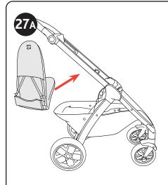
27A. Fold the bottom of the seat pad up to expose Seat Bracket. From the back of the stroller, insert the seat between the stroller frame and tilt the Seat Bracket to line up the tabs with the corresponding openings on the Seat Pan.
