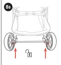
8B. Pull up on the Brake Lock Levers to unlock the Rear Wheels.
