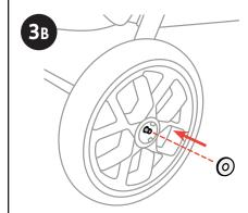
3B. On the same side, slide a Washer (E) onto the Rear Axle.
