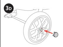
3D. Line up the tabs on the Hubcaps (G) with the holes on the Wheel. Snap the Hubcap onto the Wheel to cover the Washer and Pin. Repeat Step 3D for other side.
