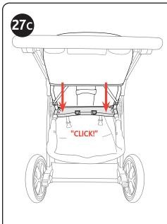
27C. Press down on the back edge of the Seat Bracket until it clicks into place, making sure both sides lock into the Stroller Frame. Then repeat steps 22-24 in reverse.
