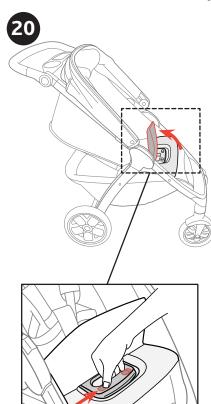
20. If attached, remove the infant car seat. Lift up the Seat Fabric and locate the Fold Handle, as shown. Slide the Handle Release button over and lift up on the Fold Handle.
