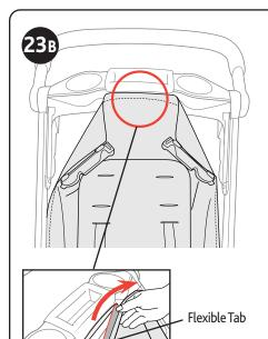
23B. The fabric will still be attached to the Parent Tray, as shown. Lift up and remove the Flexible Tab from the groove on the Parent Tray. Fold the Flexible Tab and Fabric Clips forward.
