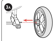
3A. On one side of the Rear Axle, slide a Rear Wheel (C), and turn the Wheel until the brake tab fits into one of the grooves on the Wheel.
