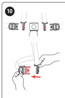
10. This stroller has a 5-point safety harness. The Shoulder Strap Connector is designed to break away from the Waist Clip when not secured in the Crotch Strap Buckle.
