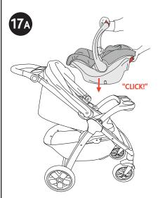
17A. With the Child's Tray attached and the Stroller Backrest FULLY RECLINED, place the Chicco infant car seat into the Stroller Frame. The car seat will only fit into the frame "REAR FACING ONLY". The baby will be facing you when pushing the stroller. Make sure infant car seat clicks into the stroller frame on both sides.
