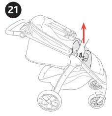
21. Pull up on the Fold Handle, the Stroller Legs and Seat back will fold down and the front wheels will automatically swivel. The closed Stroller will now stand on its wheels.
