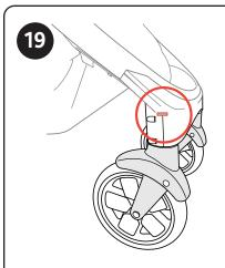
19. Remove the Front Wheels by pushing in on the Release Button, just above the wheel (as shown). And, at the same time, pull the Front Wheel off of the Stroller Frame. Repeat for the other side.
