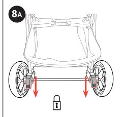
8A. Push down on the Brake Lock Levers located on each side of the Rear Wheel assembly, to lock the Rear Wheels.
