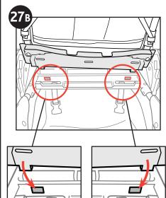
27B. Slide the tabs into the openings, to reattach the Stroller Seat .
