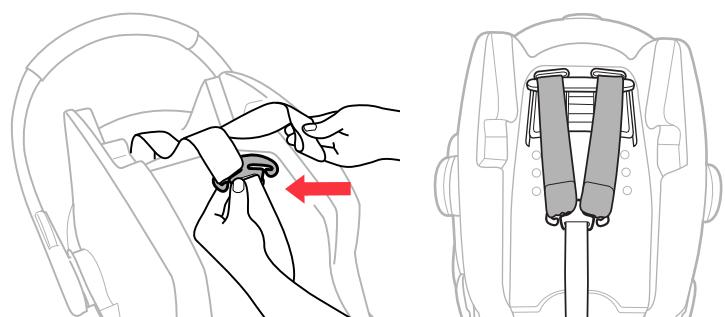
23 Flip the Carrier over and pull the harness straps through the openings. Attach BOTH Harness Straps to the Splitter Plate. Check to make sure the straps are above the Height Adjuster Plate. **WARNING - Make sure Harness Straps are not twisted and both Harness Straps are securely attached to splitter plate.**
