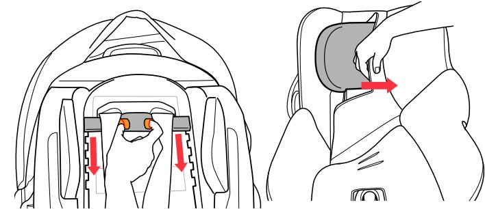
15 Adjust Head Rest to lowest position and place the seat pad onto the Carrier shell. Slide fabric opening around the Head Rest Frame.
