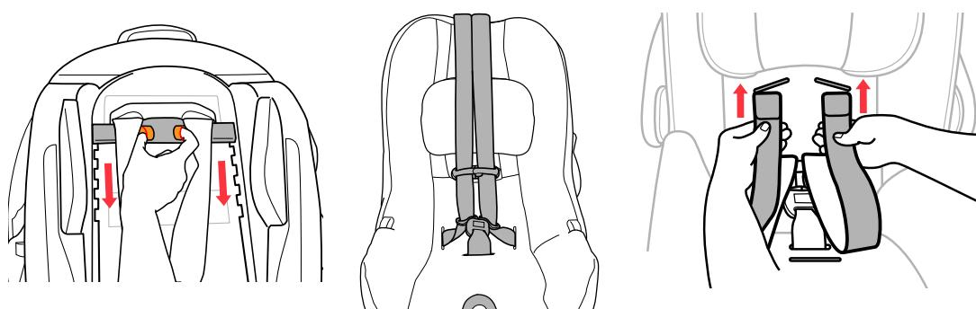
22 Make sure the Head Rest is in the lowest position. Buckle the crotch strap buckles and chest clip. Lay the Harness Straps over the seat back to make sure the Harness Straps are NOT twisted and oriented as shown. Thread Harness Strap ends into the openings on the Height Adjuster Plate.
