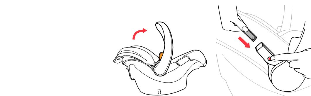
28 Rotate the Carry Handle up into the carry position. Insert one side of the Canopy bow into the Canopy Mount until it clicks, repeat for the other side. Pull on the bow on each side to check that it is securely attached. Then rotate the Carry Handle back into stationary position. Refer to User Guide if needed.
