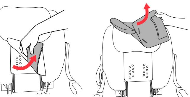
14 Adjust the Head Rest to the highest position. Attaching the Head Rest fabric, start by sliding the bottom edge of the backplate into the pocket on the back of the headrest pad. Then carefully pull both Head Rest side pockets around and over the Headrest frame.
