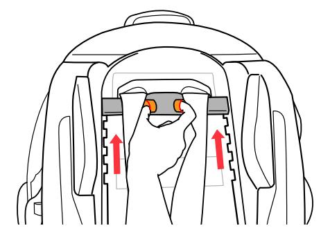
13 Adjust the headrest to the highest position. To remove the Head Rest fabric, pull down on and untuck the bottom fabric pocket from the Headrest back plate. Then guide the Headrest fabric from each side of the Headrest frame, and remove the fabric.
