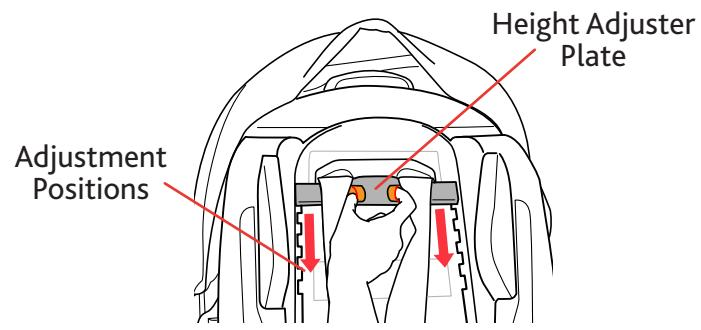
6 Flip the Carrier over and adjust Head Rest into the lowest position, using the Height Adjuster Plate.
