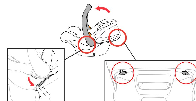
29 Re-attach the elastic straps below the Canopy Handle hub on both sides. Pull both toggles through loops on the back of Canopy. Refer to User Guide if needed.
