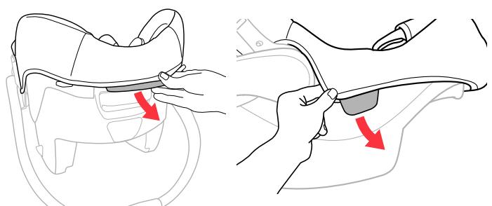
8 Place the Carrier on its side and unhook the Elastic Straps, located just below the Handle's rotating hinge. Then flip out the Plastic Tabs located below the seat belt guide. Repeat for the other side
