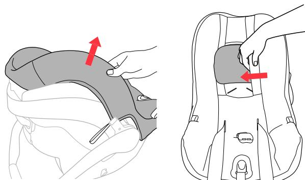
10 Pull forward on the Seat Back fabric and guide the Head Rest through the opening on the Seat Back. Pinch the Seat Pad fabric at the corner of the Harness Adjuster Strap Cover. Pull forward on the Seat Pad edge to remove the fabric from around the Harness Adjuster Strap Cover. Note: The plastic Harness Adjuster Strap Cover is NOT removable.
