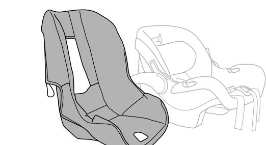
12 Remove the Seat Pad from the carrier.
