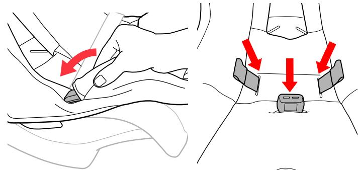
11 Slide the fabric over both seat belt guides. Feed the harness straps, chest clip sections, and crotch buckle through the fabric openings.
