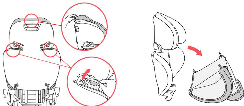
**16** Lift up on the plastic tabs at the top of the Headrest and below the Shoulder Belt Guides, as shown.
