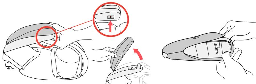
11 Locate the Armrest release button directly under the front of the Armrest. Pull on the button and at the same time lift up on the front edge to remove the Armrest cover.
