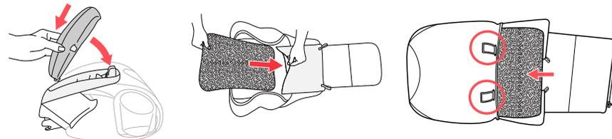
**18** Re-attach Armrest covers refer to the USER GUIDE. Repeat steps 13 thru 17 in REVERSE to attach fabric covers. Make sure to insert Foam Pad into the seat bottom. Fit fabric carefully around all orange belt guides.
