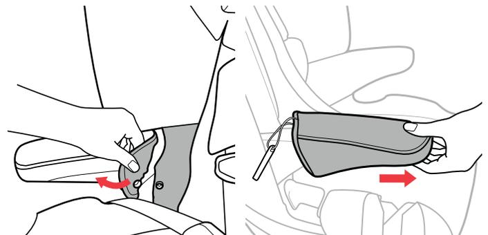
14 Undo the snap attaching the Armrest Fabric to the Backrest Seat Pad and then remove the Armrest Fabric. Repeat this step for the other Armrest.
