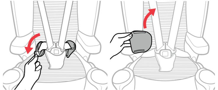
**2 Undo the hook and loop fastener on BOTH Waist Belt pads** and remove.
