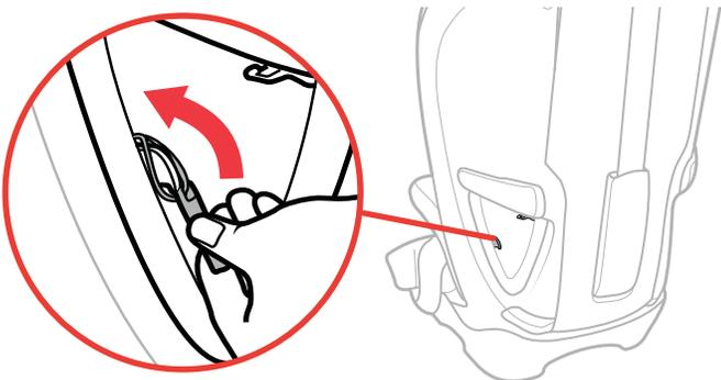
13 Unhook the Armrest fabric loop from the side hook located near the vehicle belt path. Repeat this step for the other side. **TIP:** To Assist in the removal of the Armrest fabric, push back on the fabric while removing the loop.
