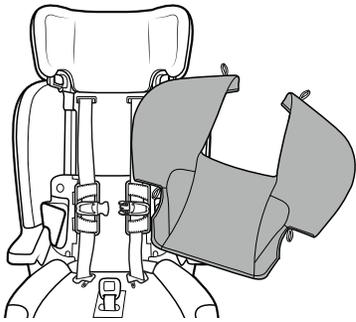
**17 Remove the Backrest Seat Pad** from the Child Restraint.
