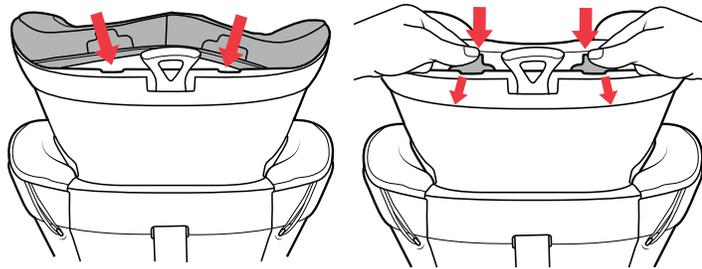
**7 Tuck the fabric into the groove at the top of the headrest.** Push down gently on both of the plastic tabs at the top of the Headrest until they snap into the grooves.
