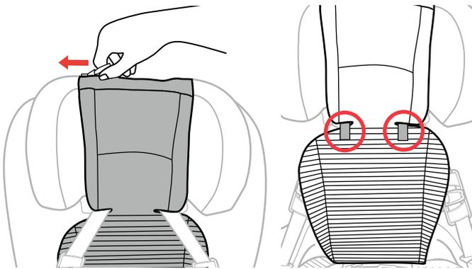
**13 Re-attach the Seat Back Air Mesh pad** by zipping the pad at the top of the headrest. Then attach both hook and loop tabs to the underside of the Headrest fabric below the Air Mesh pad.
