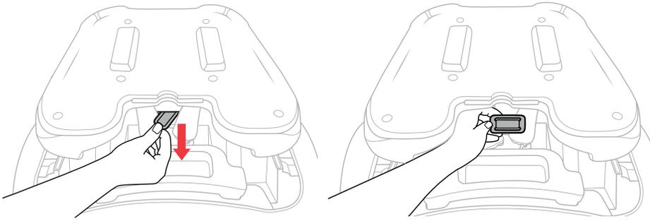
19 Push the metal bar through slot on top of the Child Restraint seat and pull through the other side. Turn the metal bar so that it lays flat on the bottom of the seat.
