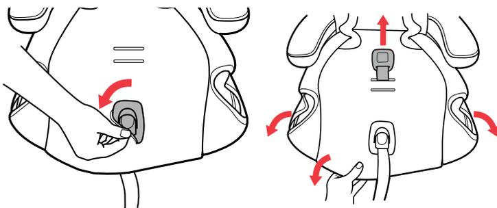
**9 Place the Seat Bottom Fabric onto the Child Restraint** and pull fabric around the Harness Adjuster Strap Cover. Then pull the Crotch Strap UP through the fabric and pull the FABRIC down and around the front and sides of the seat.
