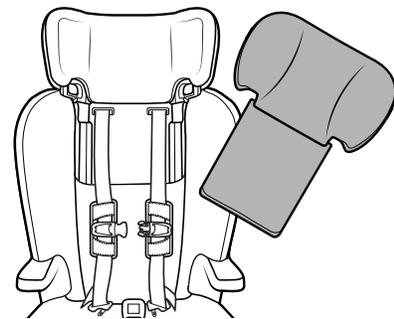
12 Remove the Headrest Fabric Pad, as shown.
