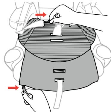
**6 Remove the Seat Bottom Air Mesh pad** by unzipping the pad at the back and front of the seat bottom. Thread the Crotch Strap down through the fabric and remove the Air Mesh Pad.
