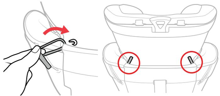
**8 With the Headrest in the highest position,** hook the elastic strap onto the **BACK** of the Headrest. Repeat this step for the other elastic strap.
