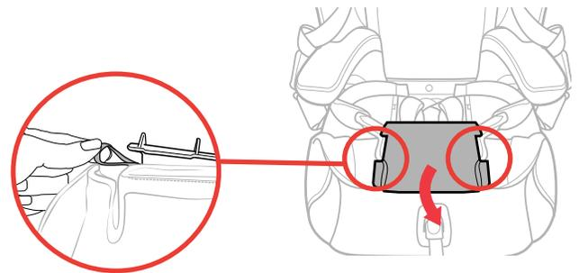
**10 Lift up on the Latch Storage Compartment door,** wrap both elastic straps on the Seat Bottom Pad around each end of the Latch Storage Compartment door, as shown. Close the Compartment door.
