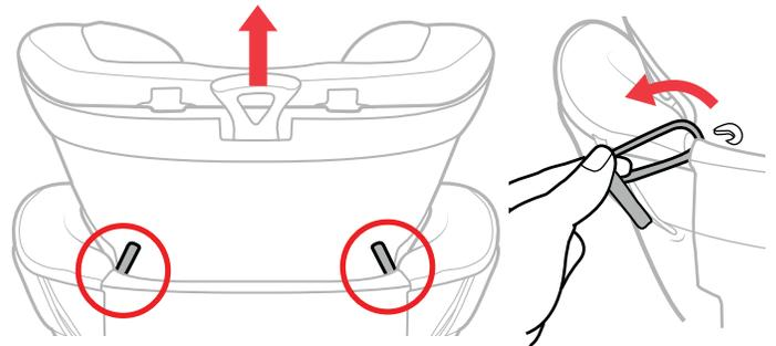
10 With the Headrest in the highest position, locate the elastic strap on the **BACK** of the Headrest and unhook by pulling up on the fabric tab. Repeat this step for the other elastic strap.
