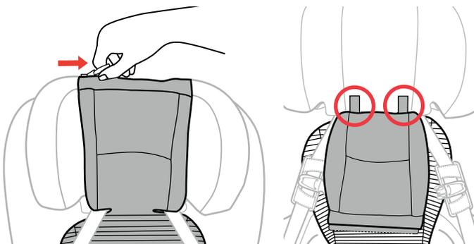
**5 Remove the Seat Back Air Mesh pad** by unzipping the pad at the top of the headrest. Then unhook both hook and loop tabs near the Shoulder Belt Guides.
