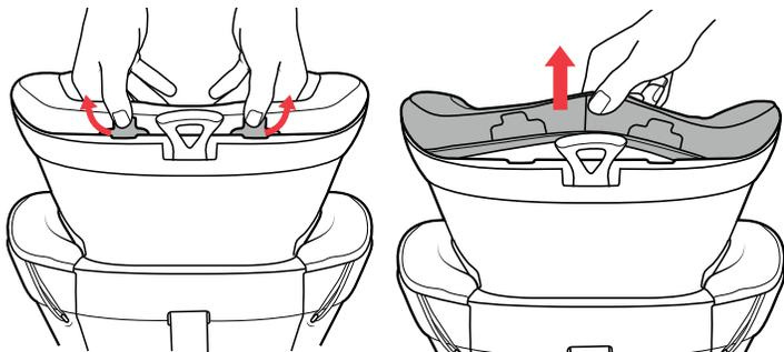
11 Pull back gently on both of the plastic tabs at the top of the Headrest and pull up on the Headrest fabric.
