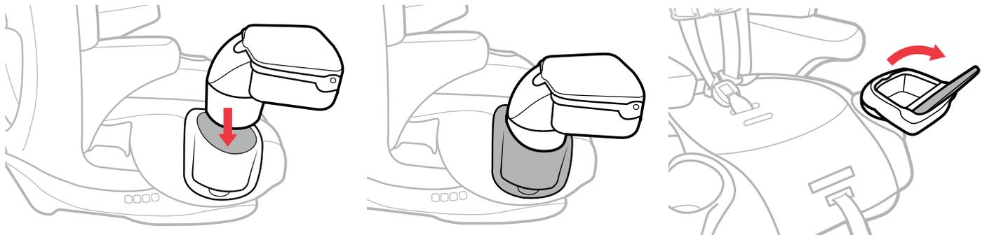
20 **Insert the console** into either of the cup holders, as shown. The KidConsole base should fit entirely inside of the cup holder. Do not force the console into the cup holder. Make sure the console fits snugly into the cup holder before use. Lift up on the tab to open the console, as shown.
