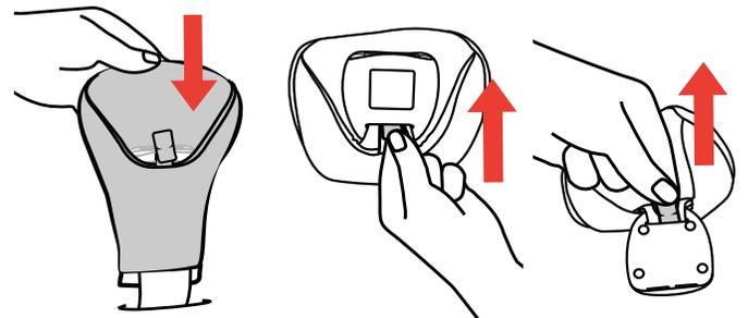
**14 Replace the Crotch Strap Pad** by sliding the Harness Buckle up through the Crotch Strap Pad. Then push the fabric Tab through the slot on the **FRONT** of the Harness Buckle. Then pull the Tab out of the **BACK** to secure it.
