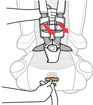
**1 Completely loosen Harness** by pressing Harness Release Button on the front of the Child Restraint and pulling out on both of the Harness Straps. Then unbuckle the Chest Clip and Harness Buckle.
