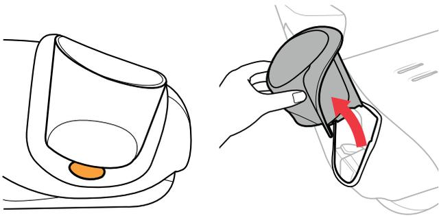
7 Remove **BOTH** of the cup holders by pressing the orange button located on the bottom edge of the Cup Holder and lifting up.
