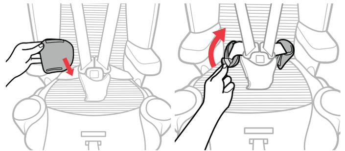
**16 To attach the both Waist Belt pads**, wrap one of the pads around the Harness Waist Strap and attach the hook and loop fasteners, repeat for the other Waist Belt pad.
