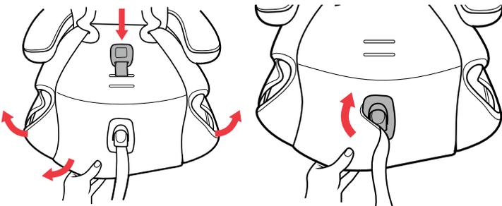
9 Thread the Crotch Strap down through the fabric and pull the **FABRIC** up around the front and sides of the seat. Then pull fabric around the Harness Adjuster Strap Cover and remove the Seat Bottom Pad. The plastic Harness Adjuster Strap Cover is **NOT** removable.
