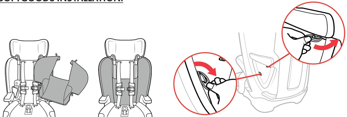
1 **Place the Backrest Seat Pad** onto the Child Restraint.
