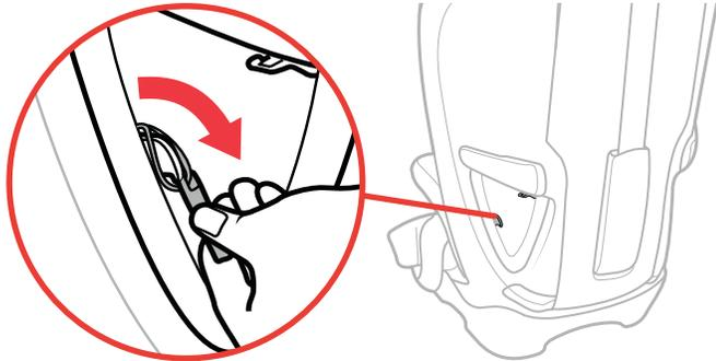
**5 Hook the Armrest fabric loop** onto the side hook located near the vehicle belt path. Repeat this step for the other side. **TIP:** To Assist in the attachment of the Armrest fabric, push back on the fabric while hooking the loop.
