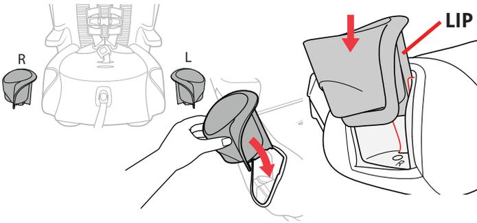
**11 Match the "R" and "L" Cup Holders** to the Child Restraint, and insert the Cup Holder. Make sure the Lip fits behind the groove and it clicks into place. Repeat this step for the other Cup Holder.
