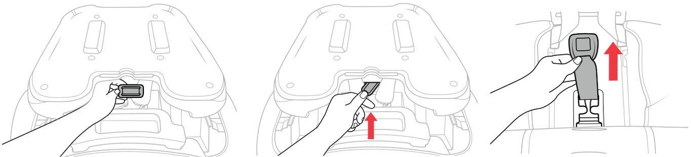
**18 Fully recline the seat** (position 1). Turn the Child Restraint over and locate the crotch strap metal bar. Turn metal bar slightly and get corner to go through slot. Push metal bar through slot while pulling crotch belt out.
