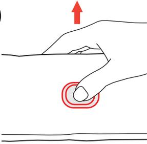
27. Lift and squeeze the Top Rails center release lock, then push down. Release all of the Top Rail locks on all 4 sides. If the Top Rail does not unlock pull up on the center hub to release the floor locks. Center floor hub must be even with top rails.
