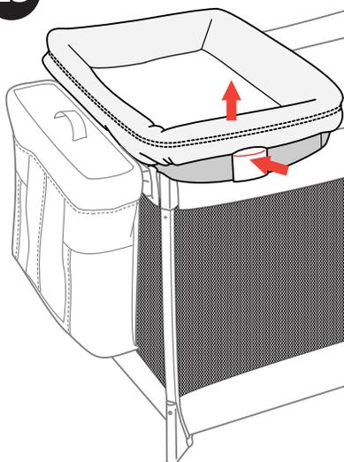
25. Remove the Changing Table by pushing in on the release buttons and lifting up.
