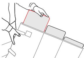
Locate the zipper on the mattress cover and unzip. Remove all of the floor boards and set them aside.
