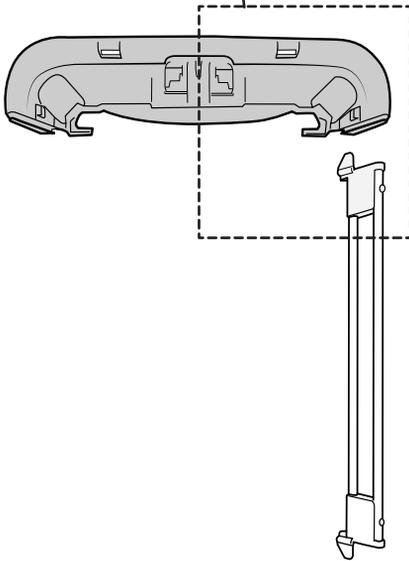
20. Slide the end of the Changing Table Frame Side into the groove of the Changing Table Frame End until it clicks into place. Make sure the tab is on the inside when assembling.
