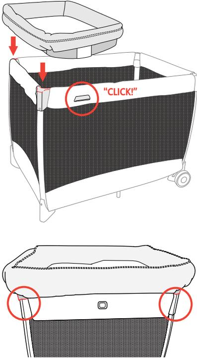
24. IMPORTANT: The Changing Table can only be attached to one end of the playard. Locate the changing table receptacles on the side of the playard. Assemble the Changing Table by lining up the corners of the changing table frame with the corners of the playard. Press down until the changing table latches into the playard receptacles. Pull up on Changing Table to check for attachment. Never use the changer on another surface or playard.
