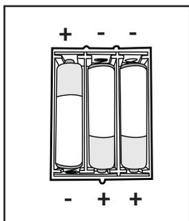
11. Before attempting to operate the Mobile unit, install 3 "AA" batteries. Use a Phillips screwdriver to unfasten battery cover and remove the battery compartment. Insert the batteries and match the polarity indicated inside battery compartment.
