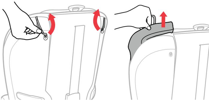
**15 Unhook BOTH elastic straps** on the back of the Child Restraint. Pull the fabric out gently from the groove around the Child Restraint. Repeat for the other side.
