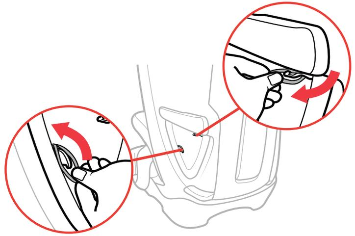
**16 Unhook the elastic strap** from the side hook and the top hook located near the vehicle belt path. Repeat for the other side.
